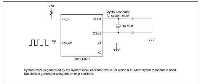
Figure 1 Subclock Operation Using On-chip Oscillator
