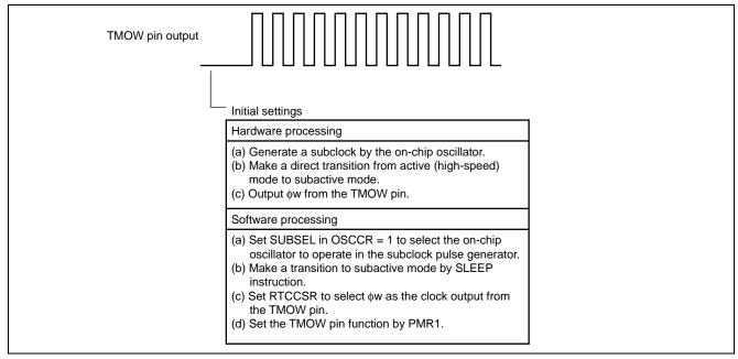
Figure 4 Subclock Operation by On-chip Oscillator
