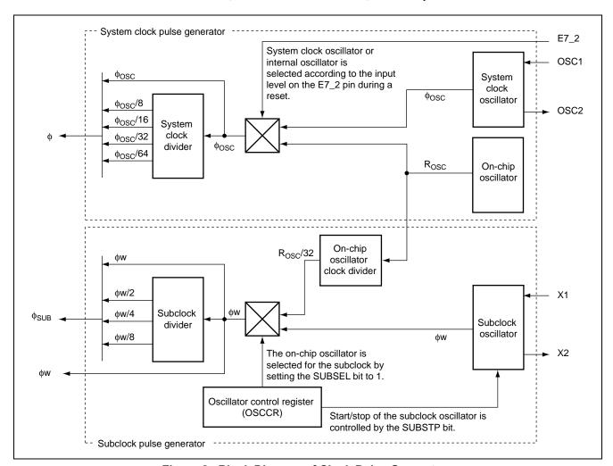
Figure 2 Block Diagram of Clock Pulse Generators
