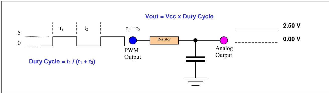
**Figure 1 Usage of PWM as D/A Converter**
