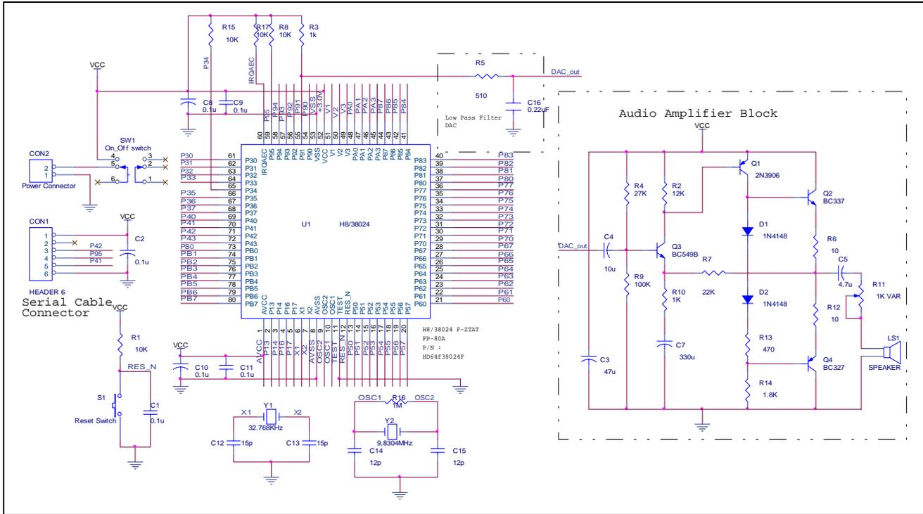
Figure 6 Schematic Diagram for PWM Tone Generator
