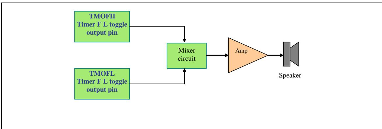
Figure 5 Block Diagram of Timer Toggle Output Tone Generator
