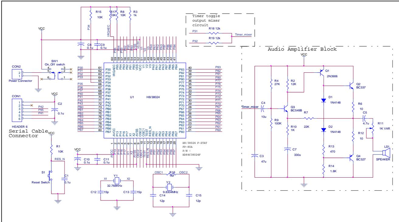
**Figure 7 Schematic Diagram for Timer Toggle Output Tone Generator**
