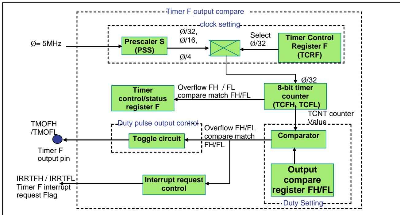
Figure 3 Block Diagram of Timer F Output Compare Operation
