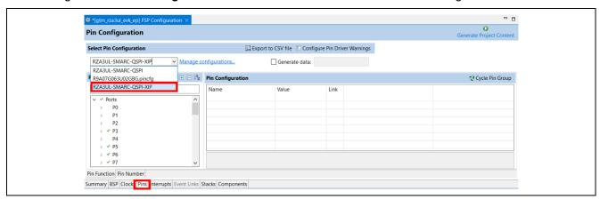
4. Check the box and enter **g\_bsp\_pin\_cfg** in **Generate data** of FSP Configuration > Pins tab.
