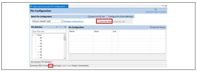
3. Change **Select Pin Configuration** to **RZA3UL-SMARC-QSPI-XIP** in FSP Configuration > Pins tab.
