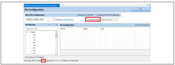
3. Change **Select Pin Configuration** to **RZA3UL-SMARC-OCTAL-XIP** in FSP Configuration > Pins tab.
