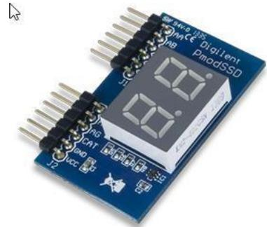
The PmodSSD utilizes a common cathode configuration to display a variety of LED segment combinations. The ten segment combinations corresponding to digits 0 - 9 are generally the most useful, although other custom combinations can also be created (see [Figure 2](#)).
