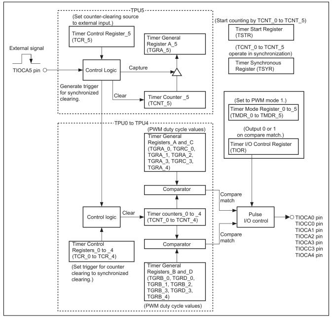
Figure 2 Block Diagram
