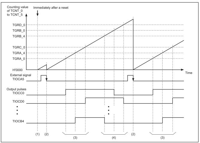
Figure 3 Operation for the Output of Pulse Signals
