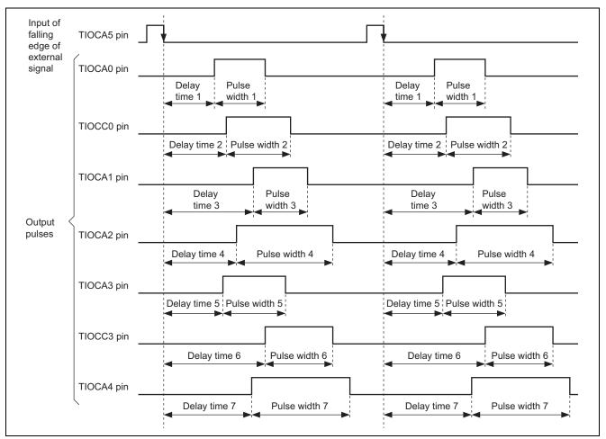
Figure 1 Example of the Output of Synchronized Pulses
