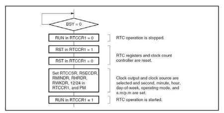
Figure 2 – Initial setting procedure
