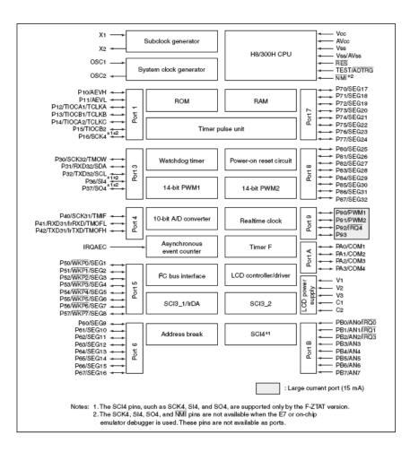
Figure 1 – H8/38076F block diagram
