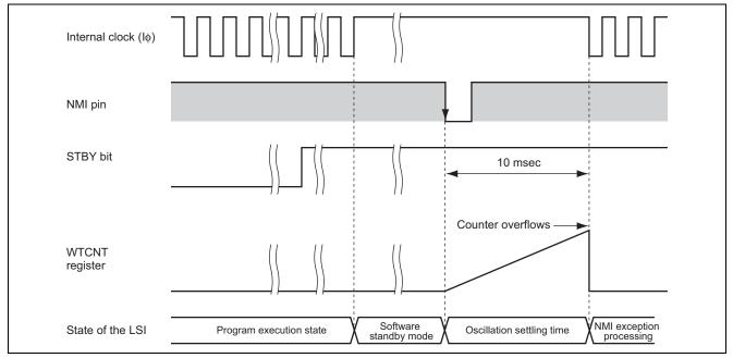
Figure 4 Timing of Sample Program Operation
