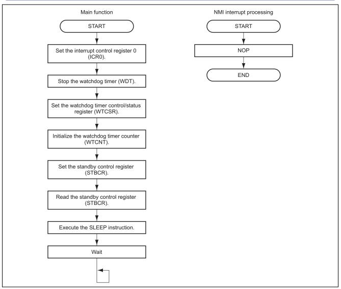
Figure 5 Flow of Processing by the Sample Program
