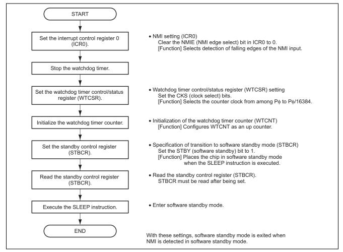
Figure 3 Setting Procedure for Entering and Exiting Software Standby Mode
