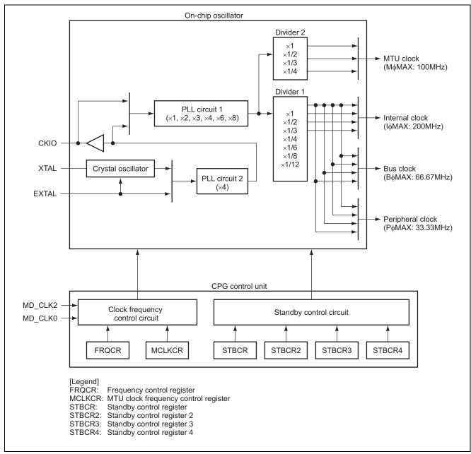
Figure 1 Schematic View of the CPG
