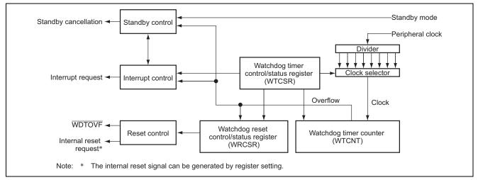
Figure 2 Schematic View of the WDT
