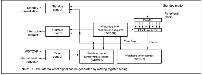
Figure 2 Schematic View of the WDT
