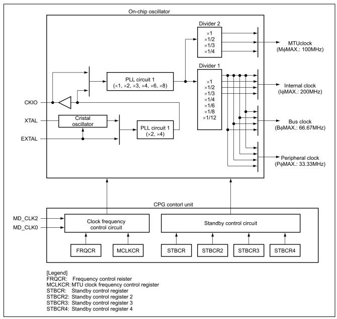
Figure 1 Schematic View of the CPG
