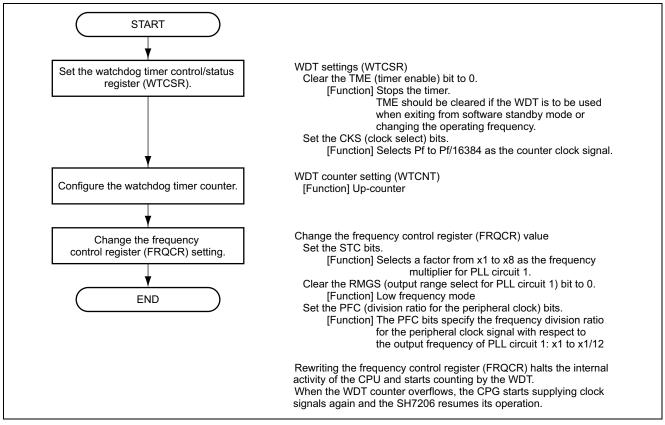
Figure 3 Example Flow for Settings to Change the Operating Frequency
