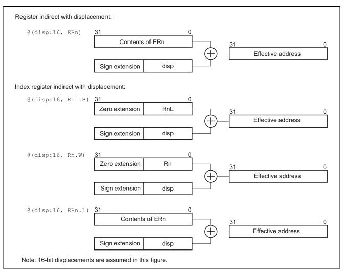
Figure 1 Calculation of the Effective Address
