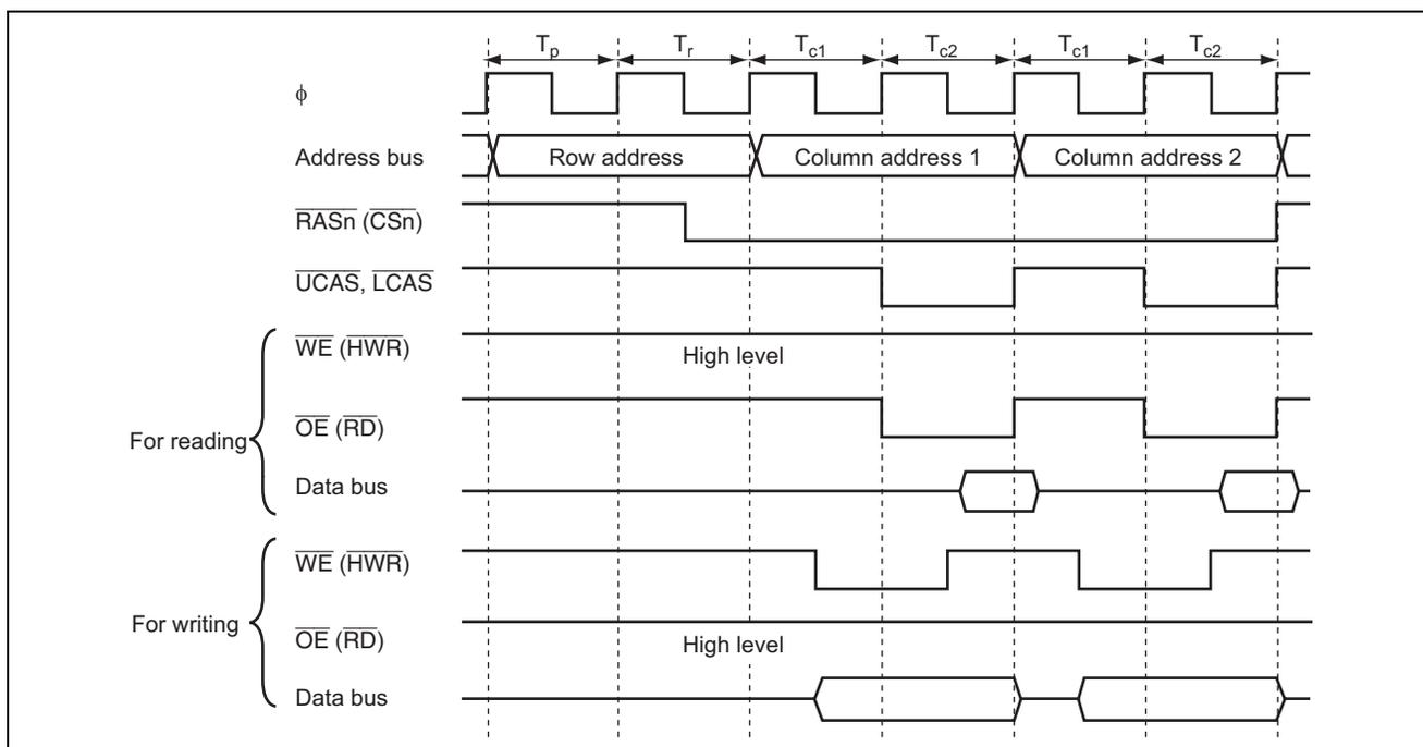
**Figure 3 Burst Mode Operation Timing**
