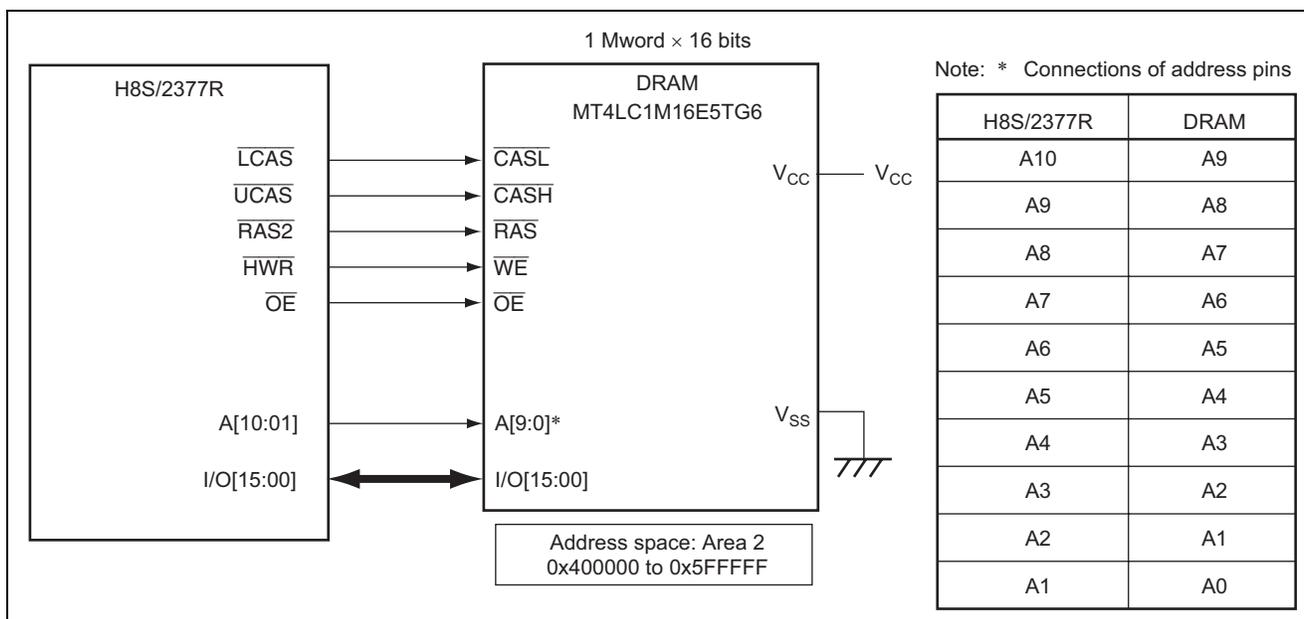
**Figure 1 Connections between H8S/2377R and DRAM**
