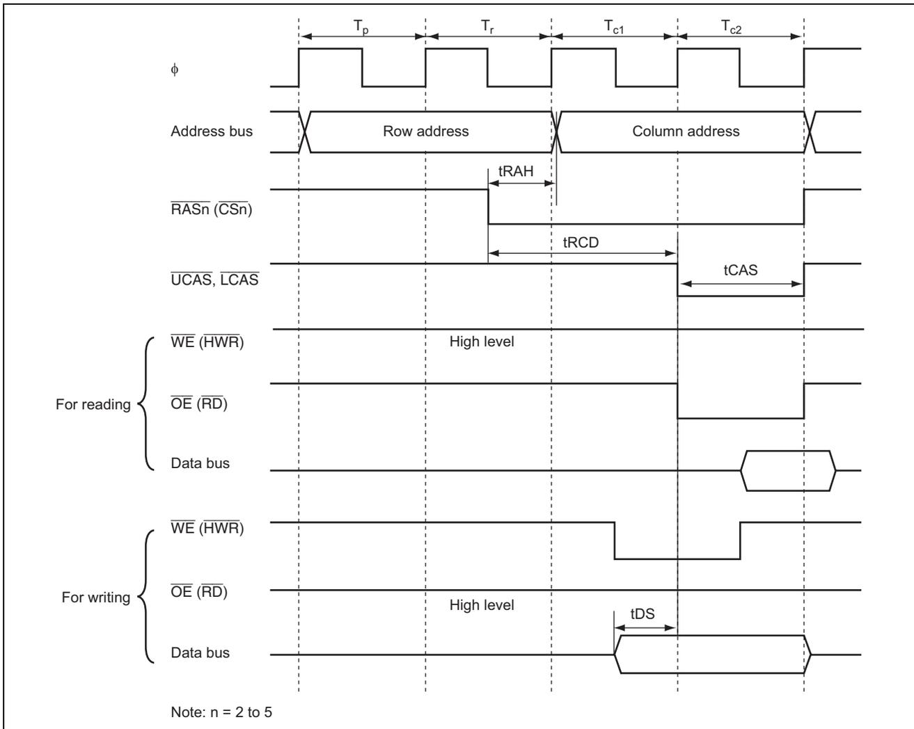
**Figure 2 Fundamental Access Timing of DRAM**
