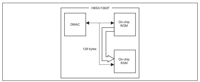
Figure 1 Transfer by DMAC
