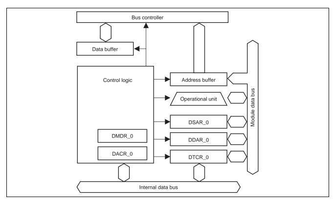
Figure 2 Block Diagram of DMAC
