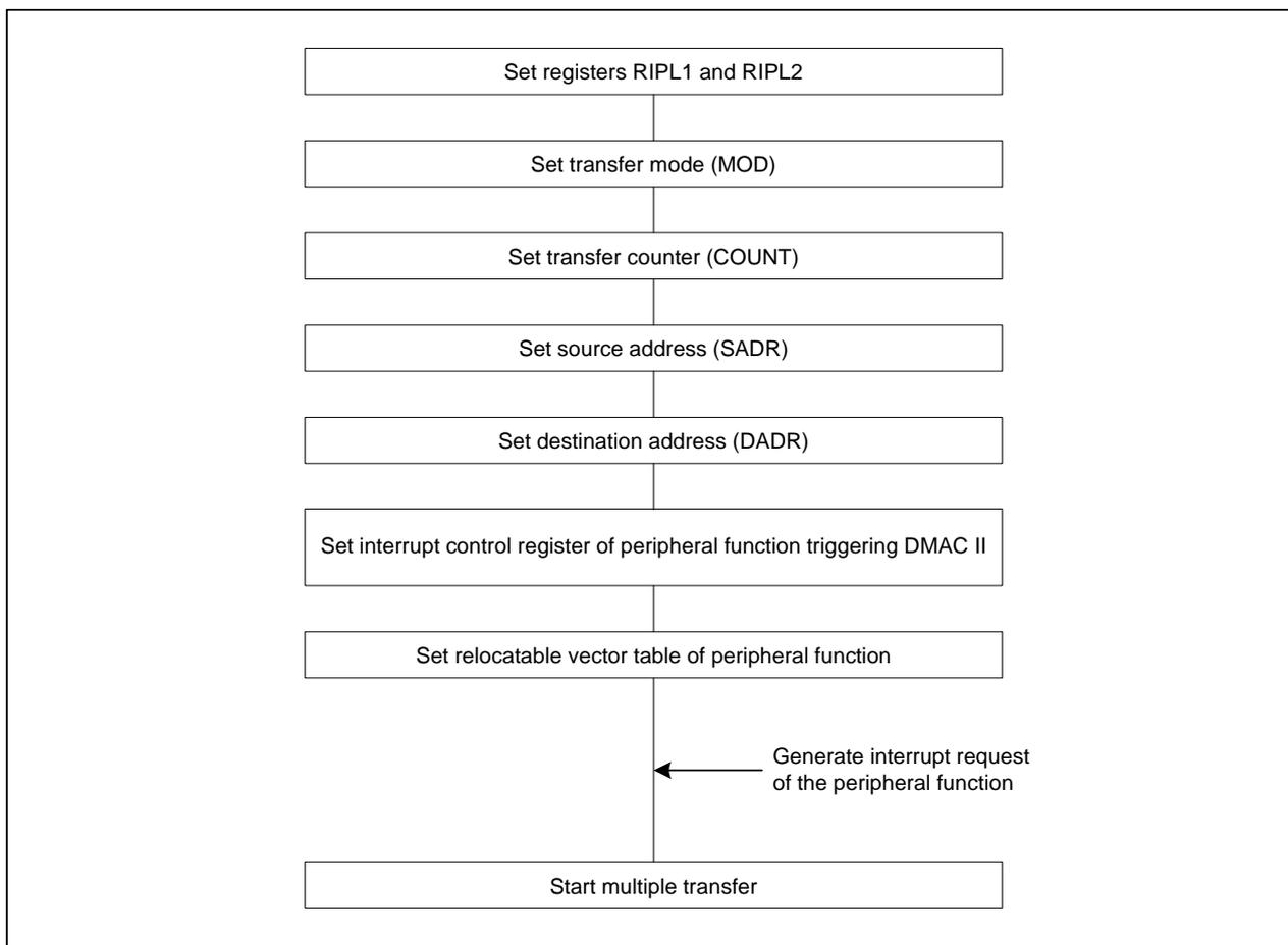
Figure 4.3 Setting Procedure for DMAC II Multiple Transfer
