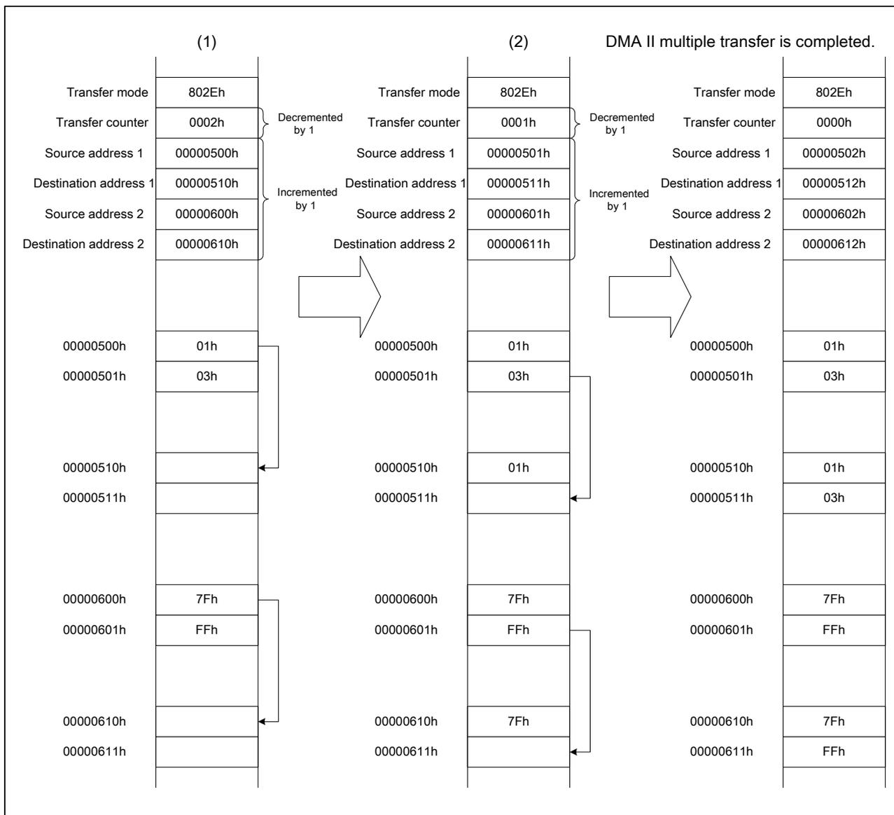
Figure 3.1 DMAC II Multiple Transfer
