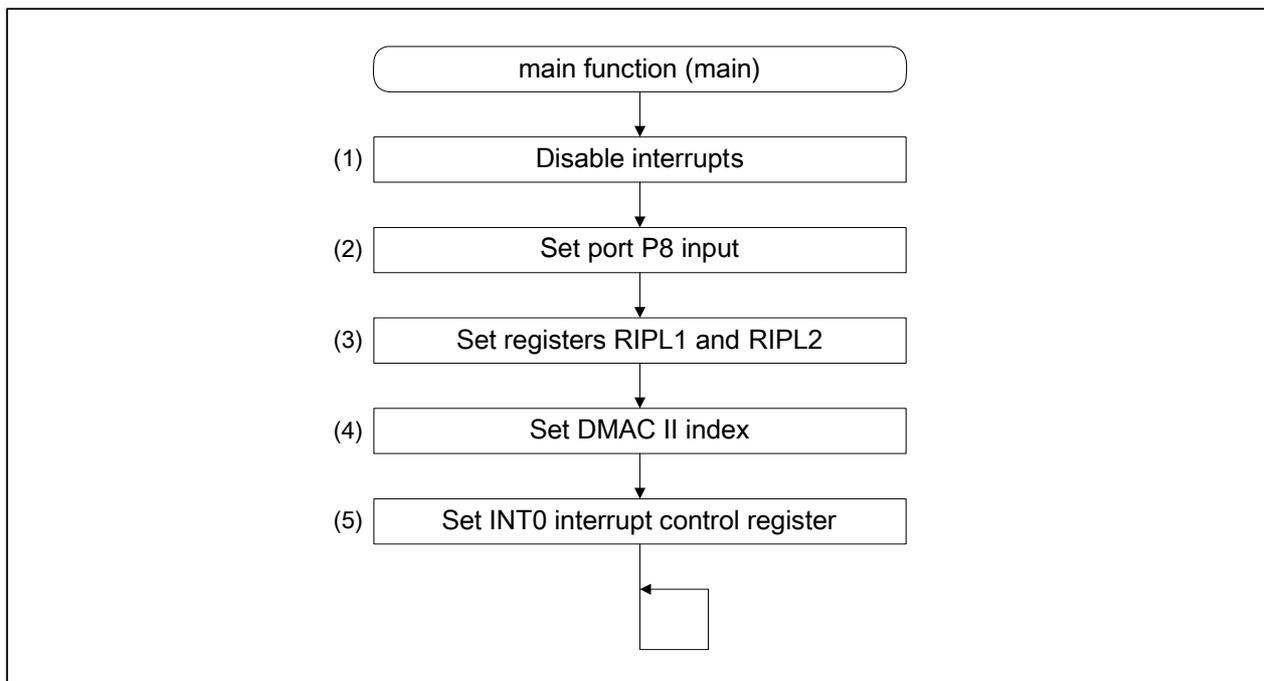
Figure 5.1 Main Function Flowchart
