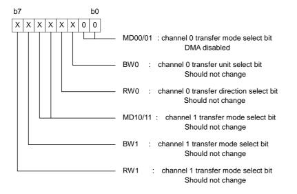
(2) Set DMA0 request cause select register (DM0SL)
