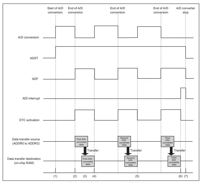
Figure 4 Timing of A/D Conversion and DTC Transfer
