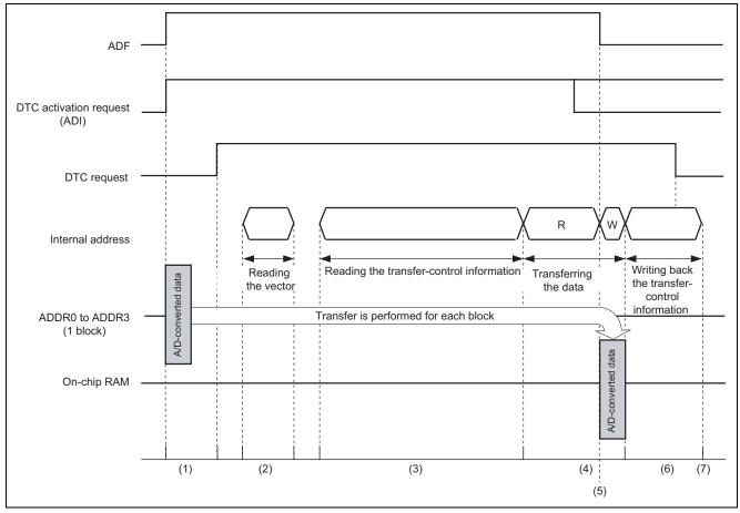
Figure 5 Detailed Timing Chart of DTC Transfer
