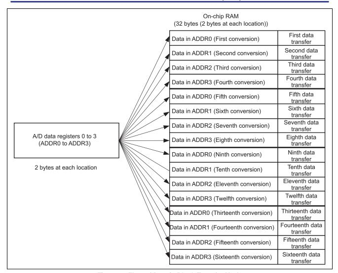
Figure 2 Flow of Data in Block Transfer Mode
