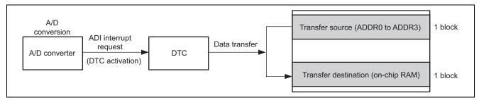
Figure 1 Overview of DTC Operation
