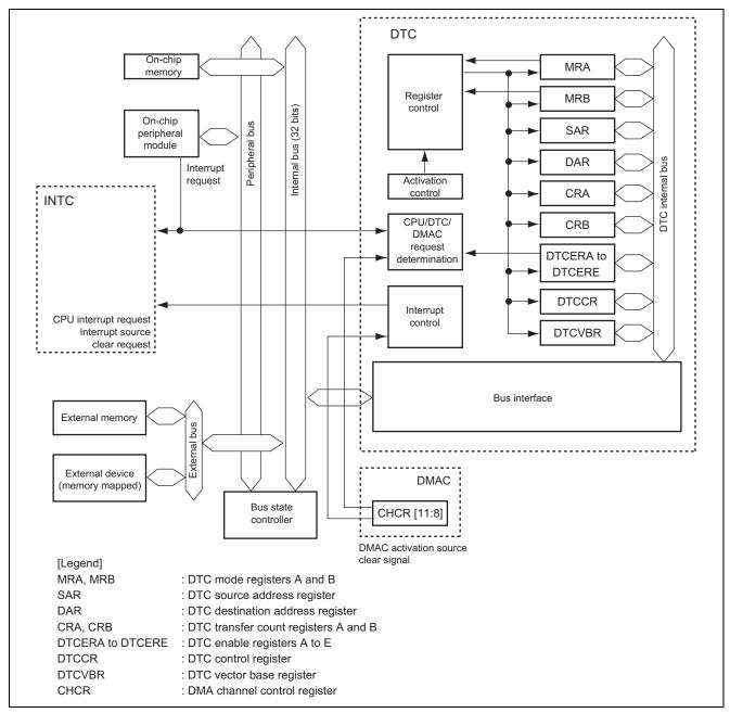
Figure 3 Block Diagram of the DTC
