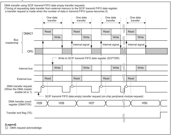
Figure 3 Operation Timing of Sample Application
