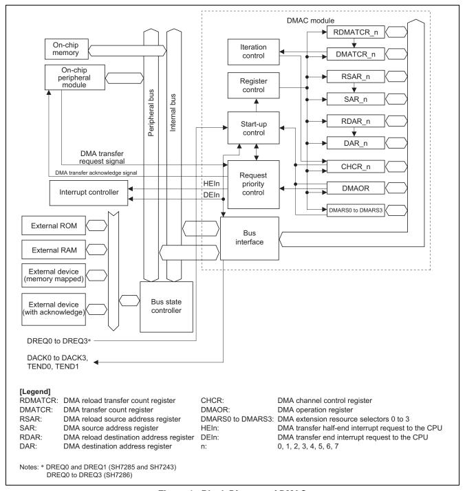
Figure 1 Block Diagram of DMAC
