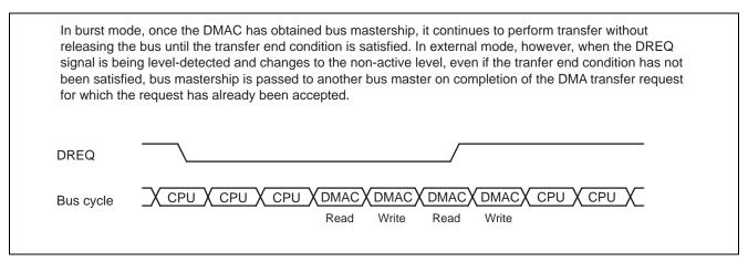
Figure 2 DMA Transfer Example in Burst Mode (Dual Address, DREQ Low Level Detection)
