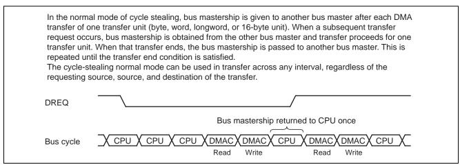
Figure 1 DMA Transfer Example in Cycle-Stealing Normal Mode (Dual Address, DREQ Low Level Detection)
