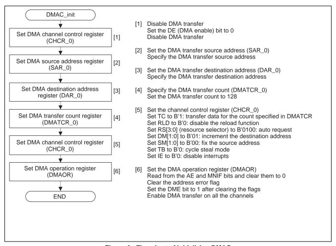
Figure 6 Flowchart of Initializing DMAC
