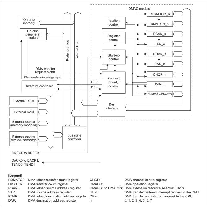
Figure 3 Block Diagram of DMAC
