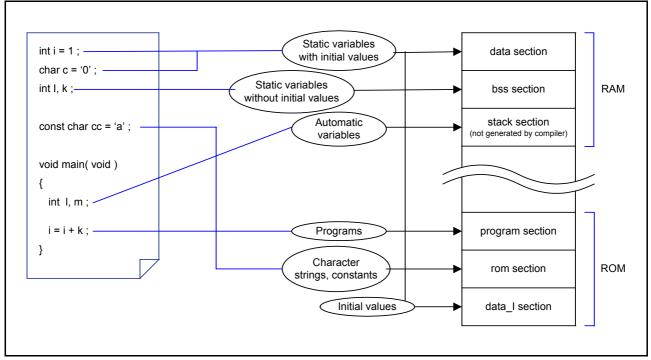
Figure 3.3 Mapping Data into Sections by Type
