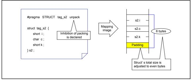
Figure 3.9 Inhibiting Packing of Struct Members
