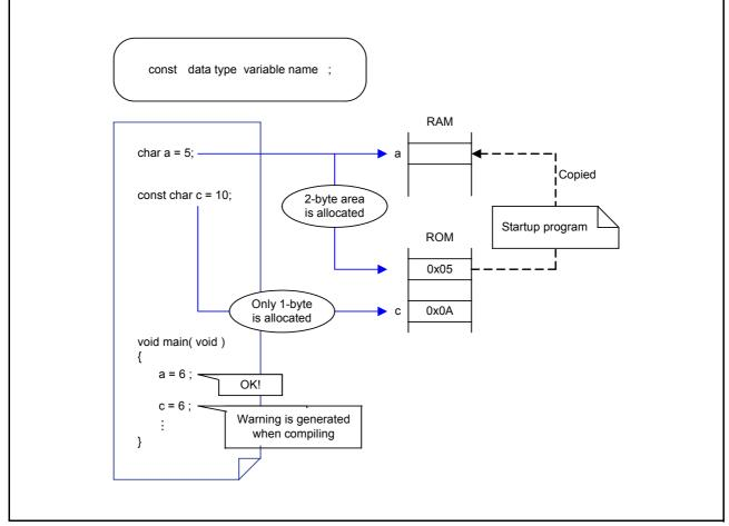
Figure 3.7 const Modifier and Memory Mapping
