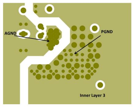
Figure 6: Inner layer 3 showing PGND and AGND
