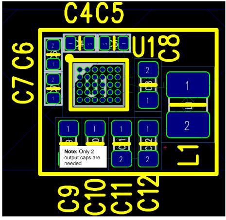
Figure 3: Components placement on Dialog's DA9155M Evaluation Board
