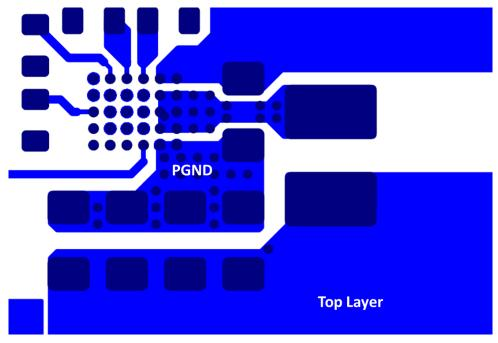
Figure 5: Top layer power ground
