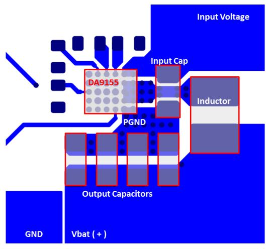
Figure 10: Output LC filter placement
