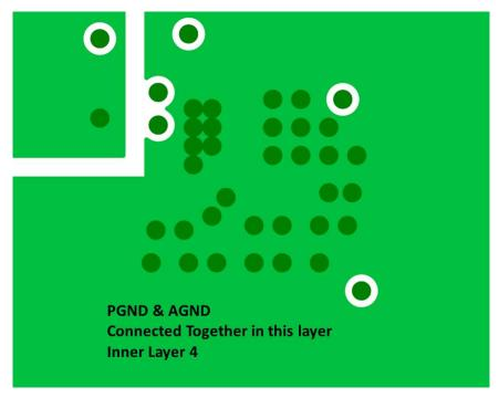
Figure 7: Inner layer 4 showing PGND and AGND
