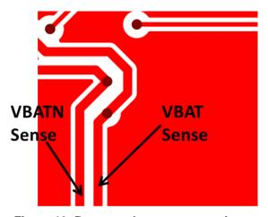
Figure 12: Battery voltage sense routing
