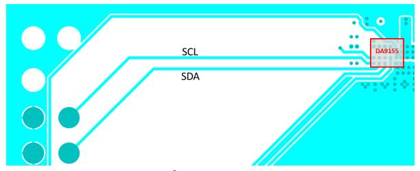
Figure 13: I<sup>2</sup>C (SDA, SCL) interface lines
