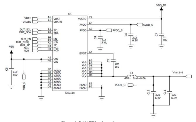
Figure 1: DA9155M schematic
