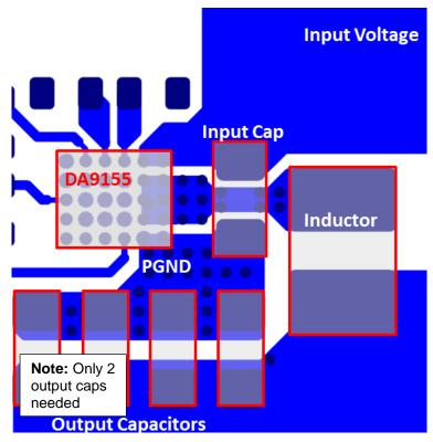
Figure 4: Recommended input capacitor placement and routing
