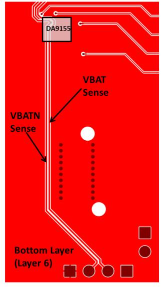
Figure 11: Battery voltage sense line routing
