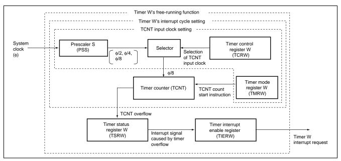
Figure 2.1 Timer W's 16-Bit Free-Running Function
