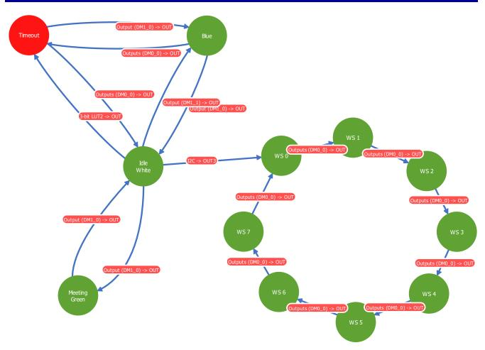
Figure 2: States of ASM of LED Indicator
