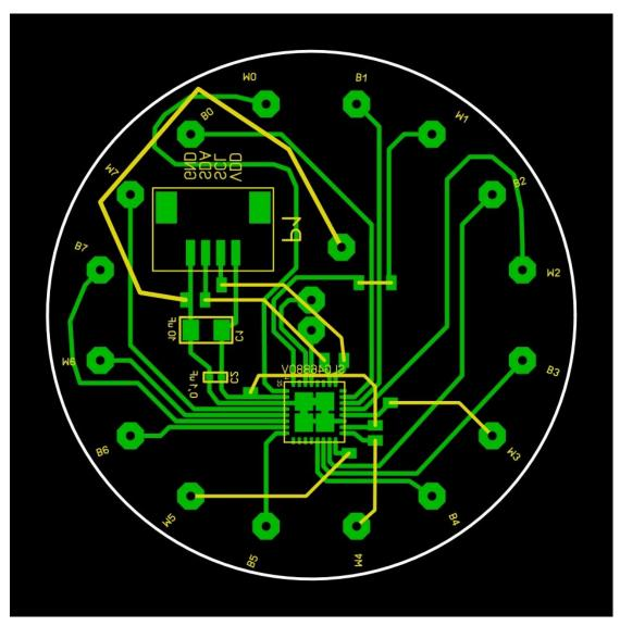
Figure 13: Top Side of PCB
