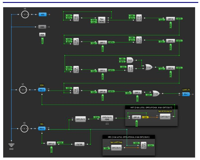
Figure 4. Smart Blind Controller Block Diagram
