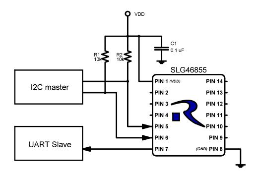
Figure 3. Block Diagram
