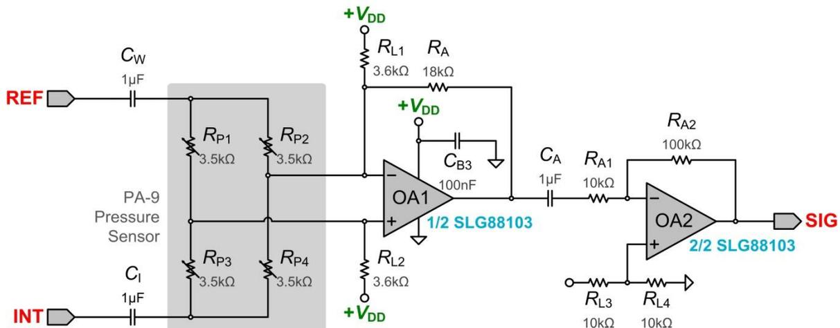
**Figure 22: Pressure Sensor with the Interfering Signal (INT)**
