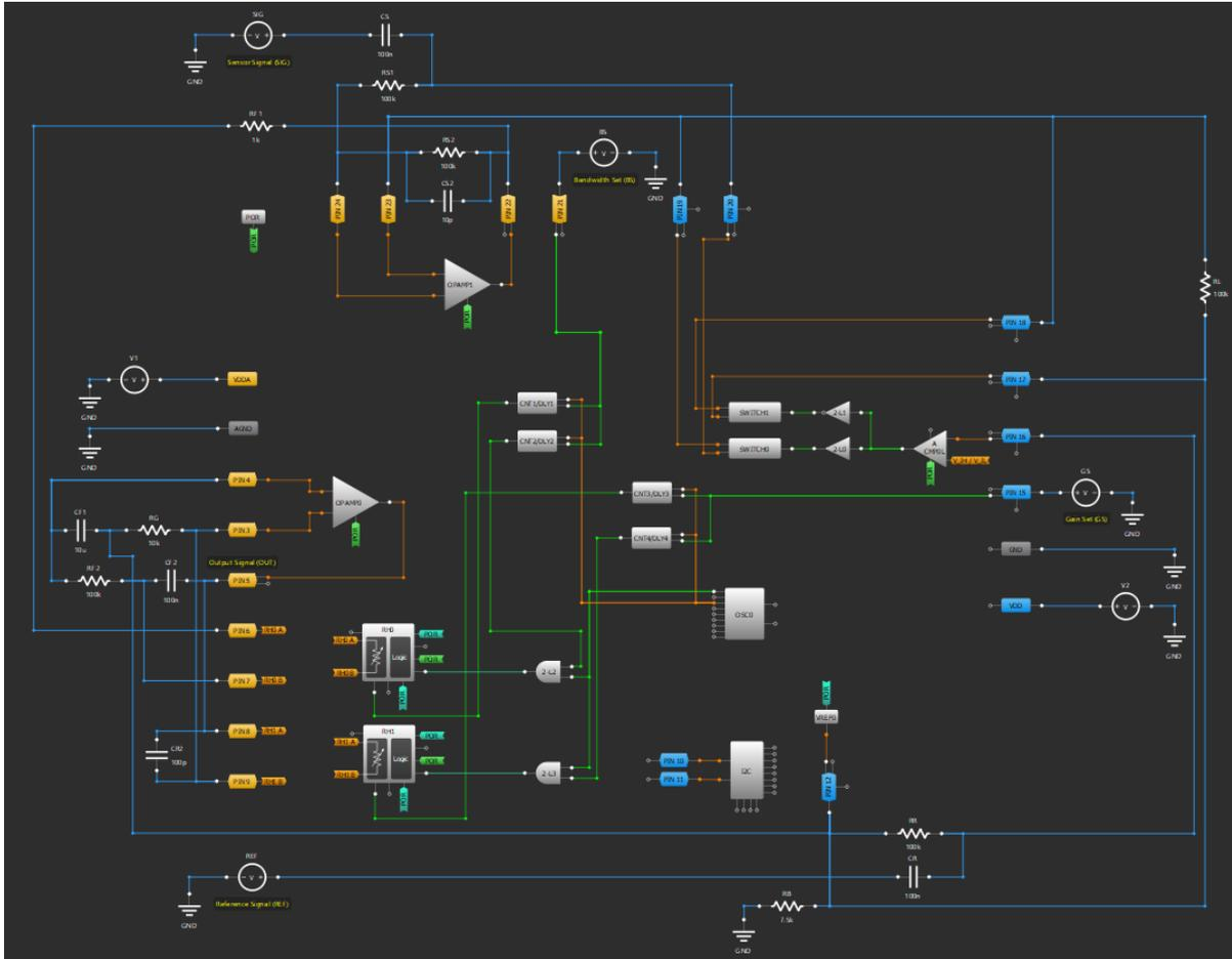
Figure 4: Lock-in Amplifier circuit in GreenPAK Designer
