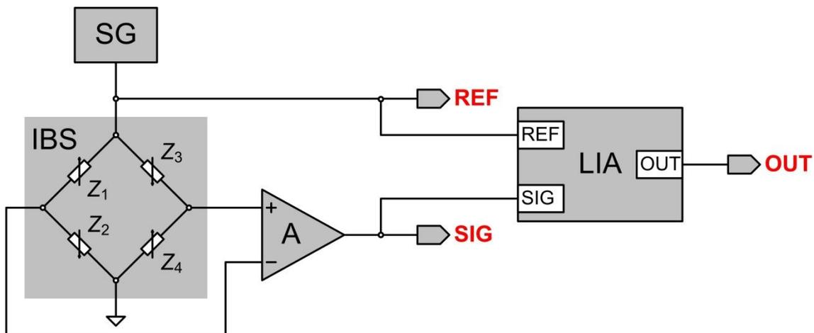
Figure 1: Typical Application of a Lock-in Amplifier
