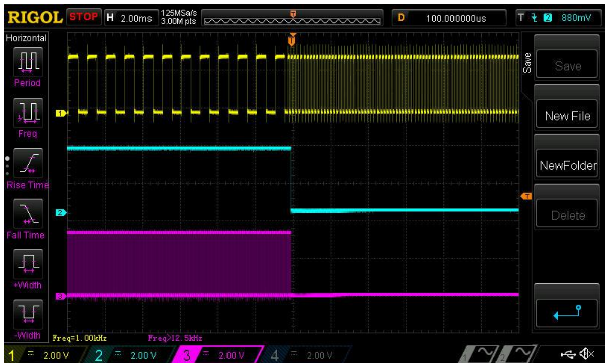
Figure 11: Waveform when input frequency is 6kHz
