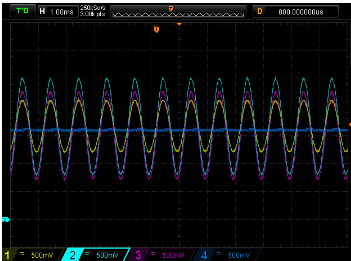
Figure 6: Waveforms after Compressing at V_{IN} = 350 \text{ mV} , R_{H0} = 1 \text{ k}\Omega , R_{H1} = 8 \text{ k}\Omega (Gain = 2)
