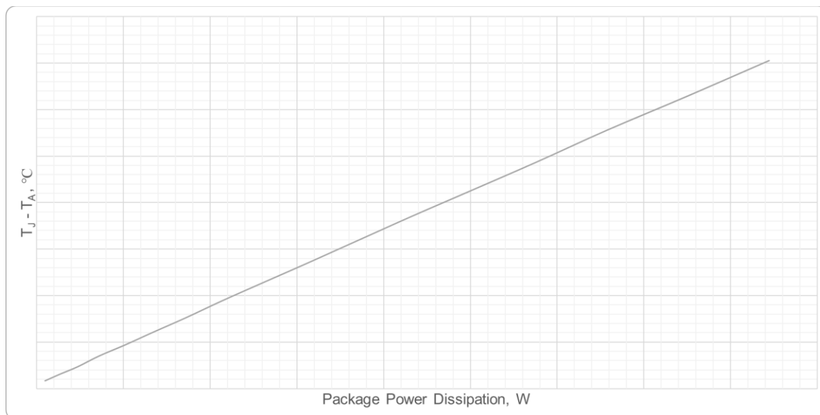
Figure 4. Plotting of Package Power Dissipation vs. \Delta T to Obtain Thermal Resistance
