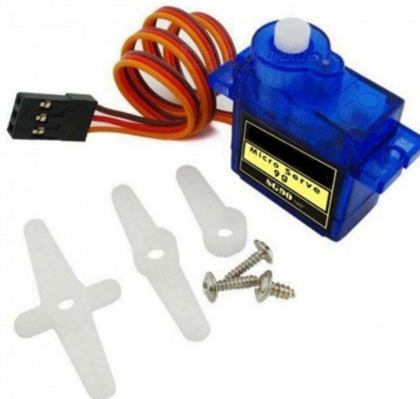
Figure 1: SG90 Model Servo Motor
