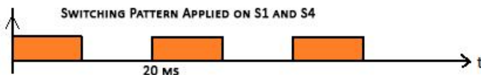
Figure 3: Switching Pattern for S1 and S4
