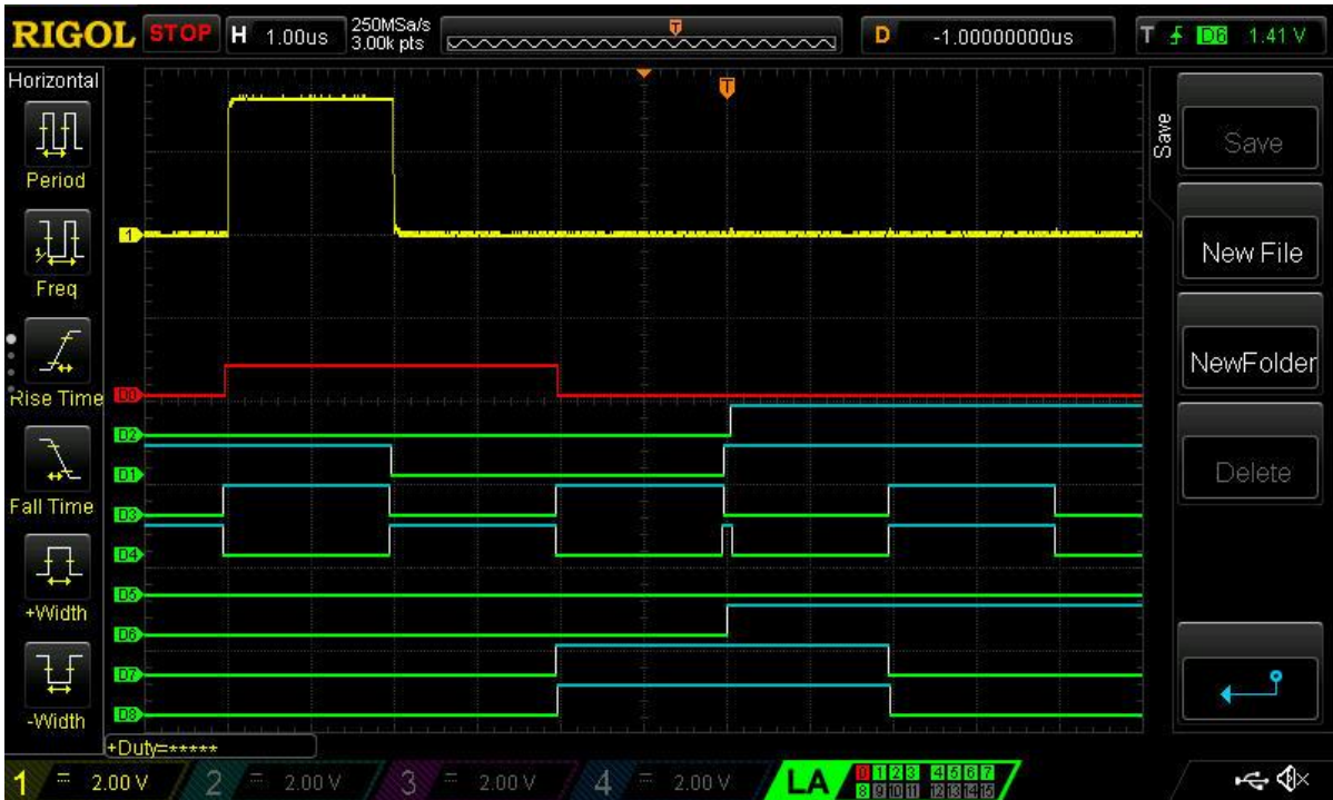
Figure 9: Duty Cycle Becoming Minimum
