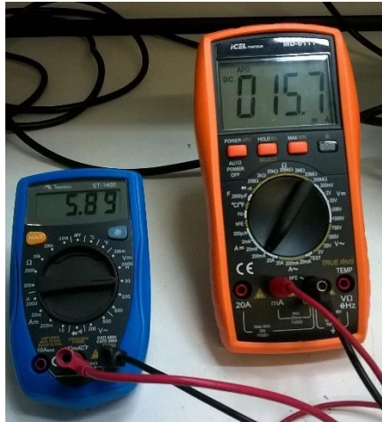
Figure 13: Measurement of Input Current and Output Voltage with a Light Load
