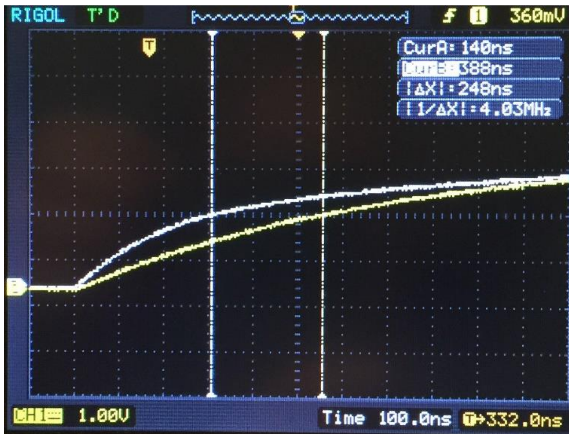
Figure 2: Oscilloscope Capture Showing the Difference in Risetime
