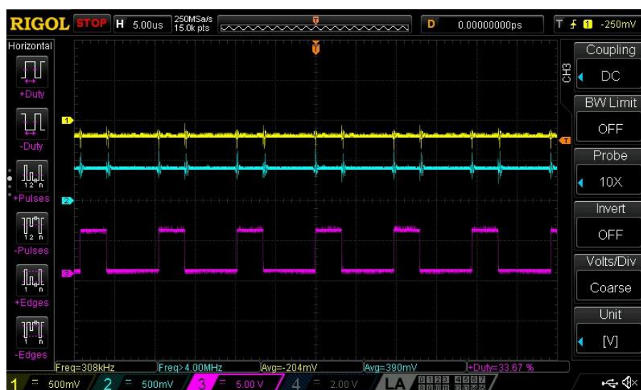
Figure 13: 30% Output Duty Cycle, ANALOG_IN \approx 400 mV
