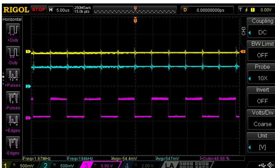
Figure 12: 50% Output Duty Cycle, ANALOG_IN \approx 550 mV
