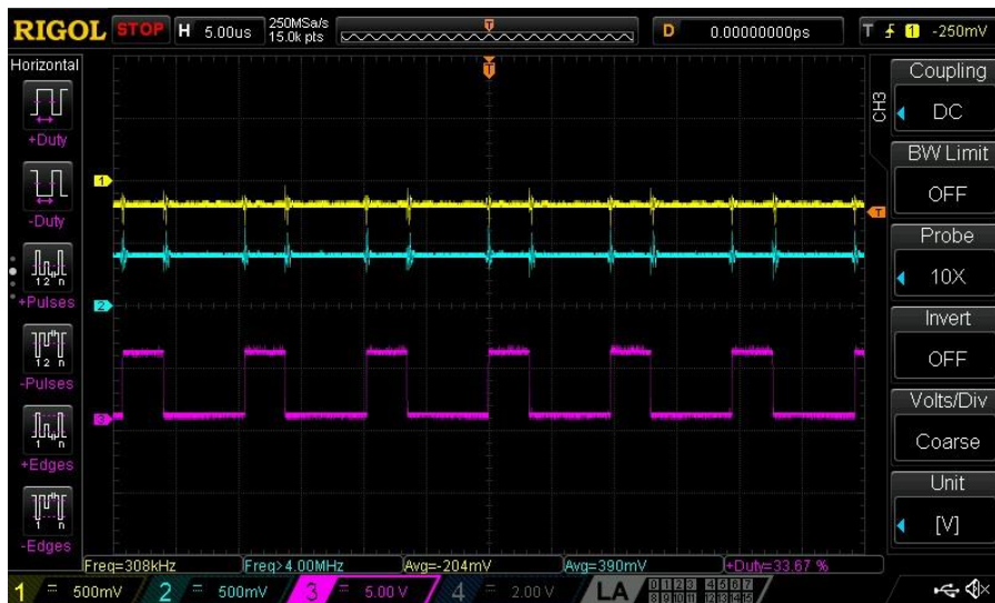
Figure 13: 30% Output Duty Cycle, ANALOG_IN \approx 400 mV
