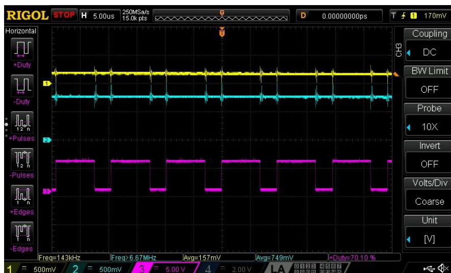
Figure 11: 70% Output Duty Cycle, ANALOG_IN \approx 700 mV
