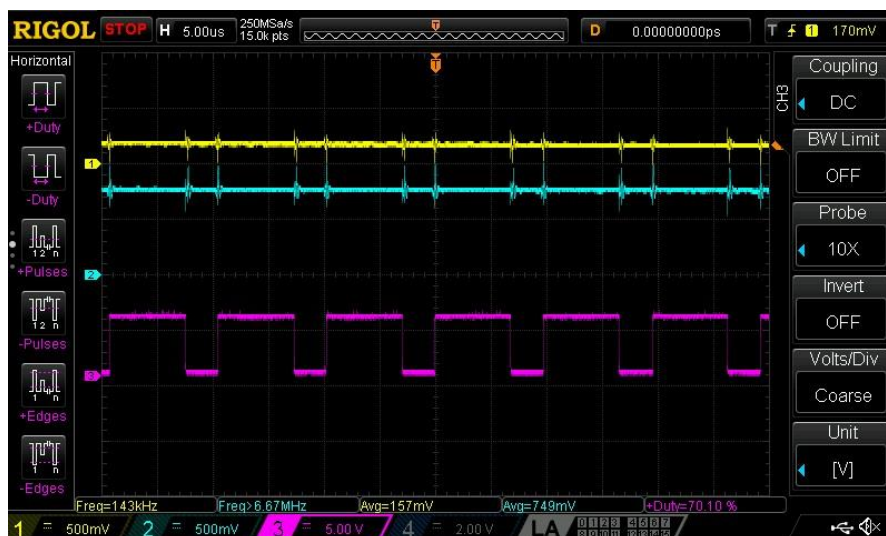
Figure 11: 70% Output Duty Cycle, ANALOG_IN ≈ 700 mV
