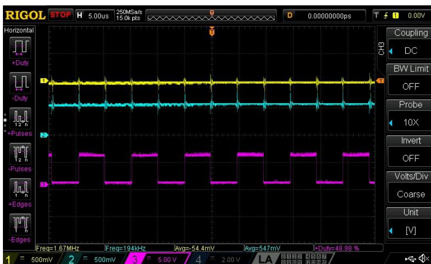
Figure 12: 50% Output Duty Cycle, ANALOG_IN ≈ 550 mV
