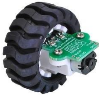
Figure 3: Pololu Wheel Encoder, Motor and Wheel
