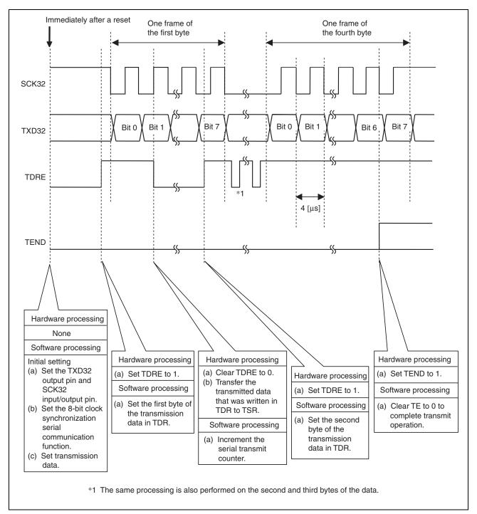
Figure 3 Operation during Transmission of Data
