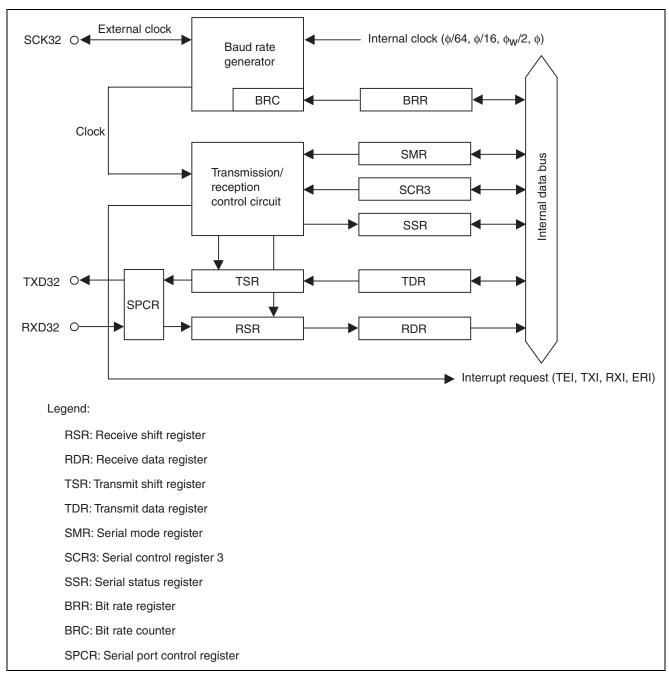
Figure 2 Block Diagram of SCI3
