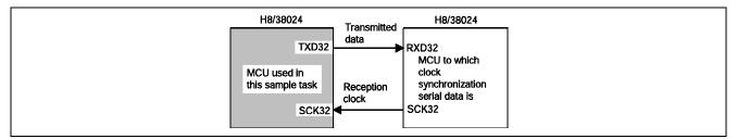
Figure 1 Clock Synchronization Serial Data Slave Transmission with the H8/38024
