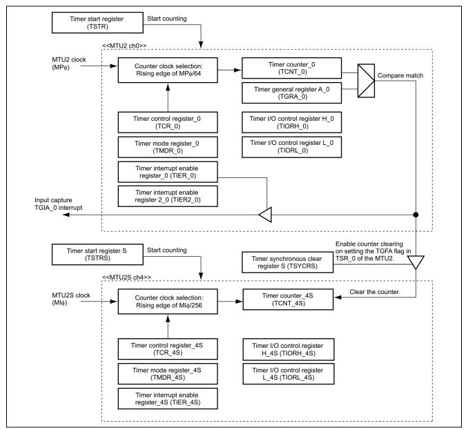
Figure 2 Operational Block Diagram of Channel 0 of MTU2 and Channel 4 of MTU2S
