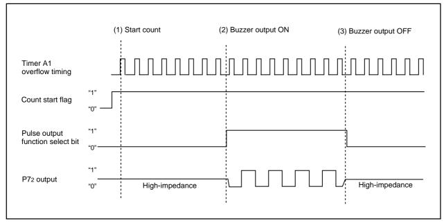
Figure 1. Operation timing of buzzer output
