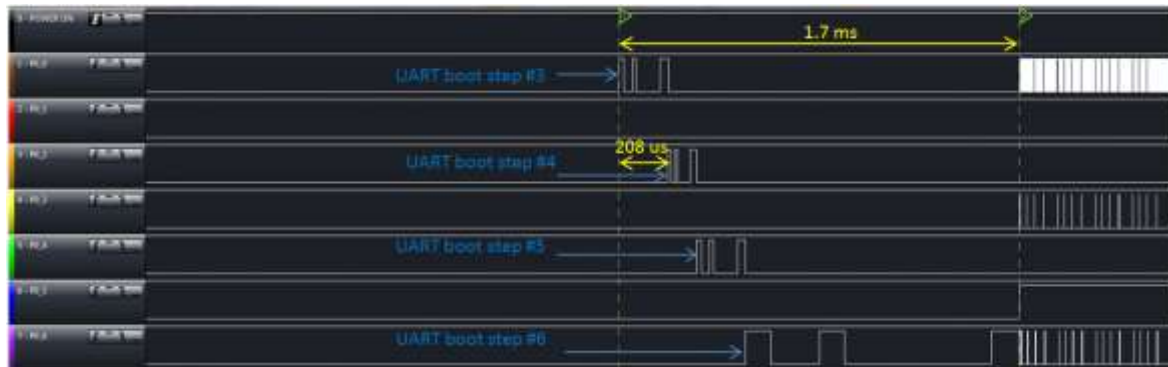
Figure 7: Boot timing from UART
