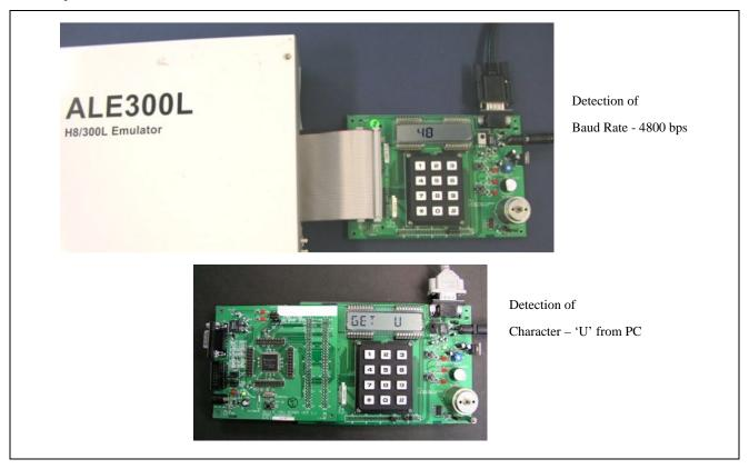
Figure 2 Use of ALE300L Emulator or SLP CPU Board with the General Application Board
