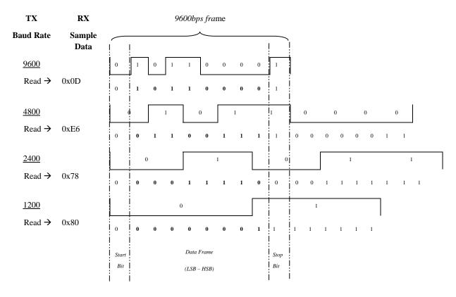
The transmitter's serial data stream, which based on different baud rate will be fed into the 9600bps receiver. Data will be sampled at this rate. With the first data bit being the least significant bit.
