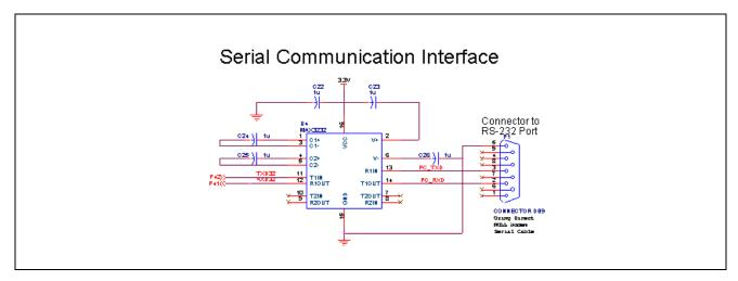
Figure 3 RS232 serial connection
