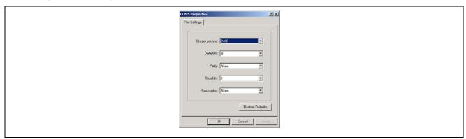
Figure 4 PC HyperTerminal setting
