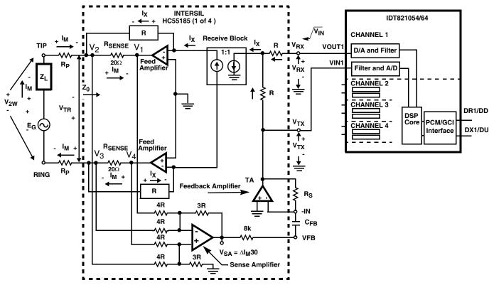
FIGURE 2. HC55185 SIMPLIFIED AC TRANSMISSION CIRCUIT AND IDT821054/64
