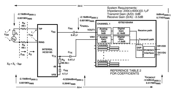
FIGURE 6. REFERENCE DESIGN OF THE HC55185 AND THE IDT821054/64 WITH CHINA COMPLEX LOAD IMPEDANCE
