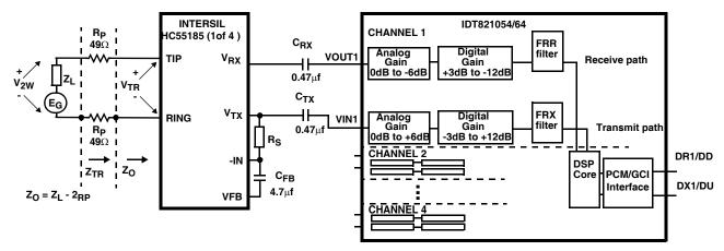
FIGURE 3. RECEIVE GAIN G(4-2), TRANSMIT GAIN (2-4)
