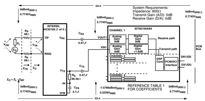
FIGURE 5. REFERENCE DESIGN OF THE HC55185 AND THE IDT821054/64 WITH A 600 $\Omega$  LOAD IMPEDANCE
