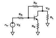
FIGURE 6. SINGLE STAGE SHUNT AND SERIES FEEDBACK CIRCUIT
