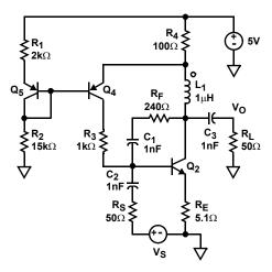
FIGURE 7. WIDEBAND AMPLIFIER REALIZED WITH HFA3096
