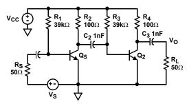
FIGURE 2. HIGH-GAIN LOW-NOISE AMPLIFIER REALIZED WITH HFA3127
