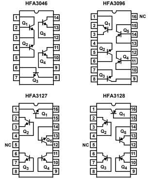
FIGURE 1. PINOUTS OF HFA3046/3096/3127/3128 SOIC PACKAGED TRANSISTOR ARRAYS
