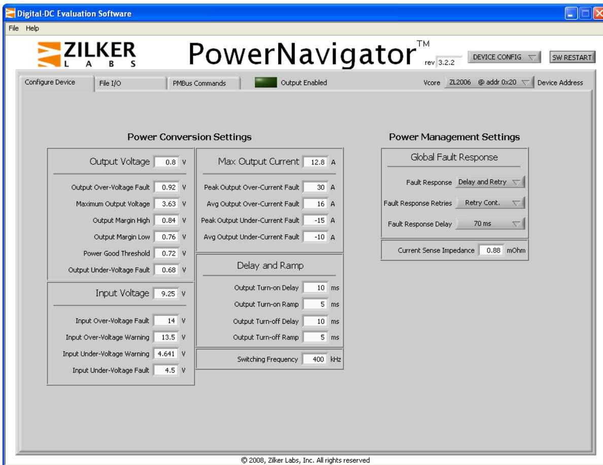
Figure 2. DEVICE CONFIG screen: Configure Device tab
