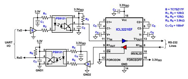
Figure 7. 3.75kV Isolated RS-232 Interface
