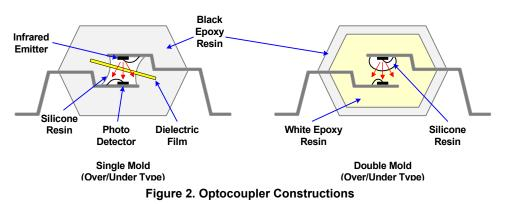
The single molded over/under technique provides the best light coupling efficiency because a silicone resin is used as a medium for direct contact between the LED and the Si detector die. To further improve the common-mode noise rejection and isolation voltage, glass or polyamide film is inserted in between the LED and the detector die. A black epoxy resin is used to house the device.
