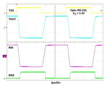
Figure 8. Signal Waveforms for Transmit and Receive Channels
