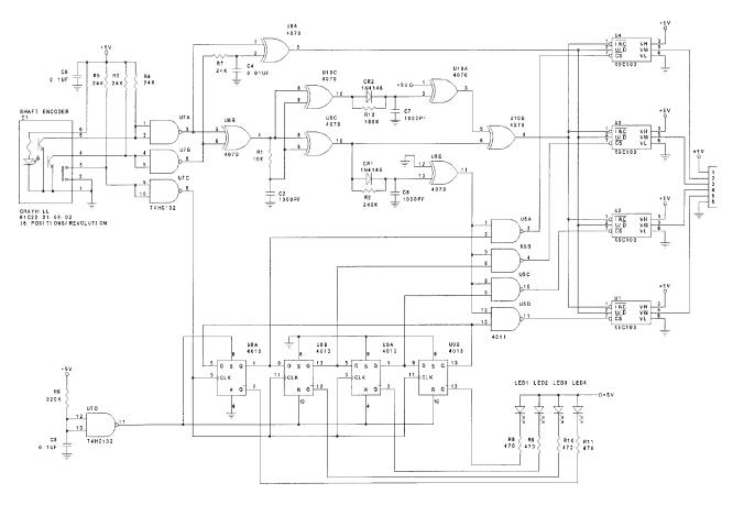
FIGURE 1. SHAFT ENCODER DRIVING MULTIPLE XDCPs
