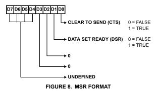
**D0 – Clear to Send (CTS).** This is both a status and control signal from the modem. It tells the 82C52 that the modem is ready to receive data from the 82C52 transmitter output (SDO). If this line is inhibited (false), then the 82C52 will not be able to begin transmission of data. Should this line go false in the middle of a transmission, the UART will only be able to finish transmission of the current character.
