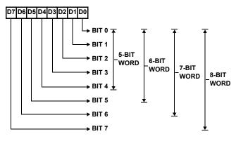
NOTE: THE LSB, BIT 0 IS THE FIRST SERIAL DATA BIT RECEIVED FIGURE 10. RBR FORMAT
