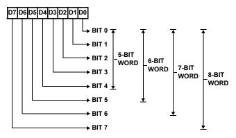
NOTE: THE LSB, BIT 0 IS THE FIRST SERIAL DATA BIT TRANSMITTED
