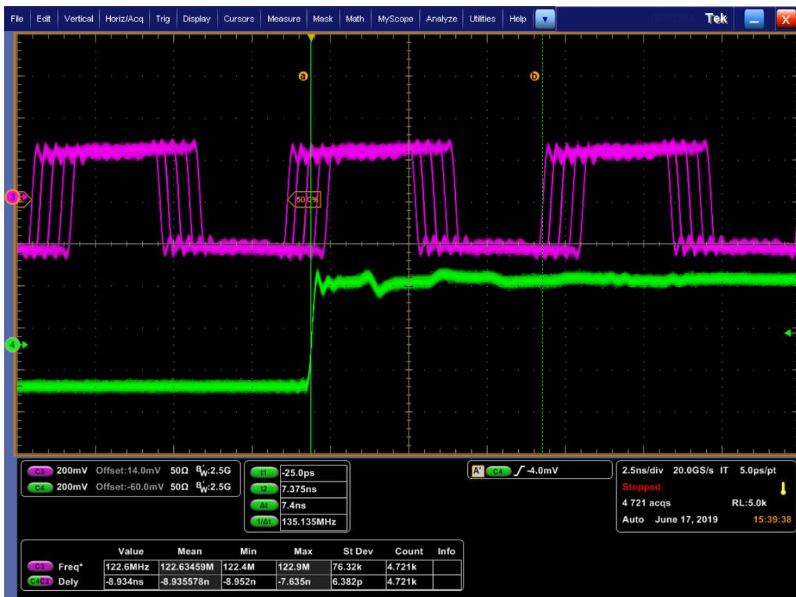
Figure 3. Result of Adjusting Individual Sysref Phase Delay
