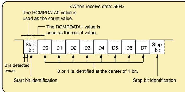
The identification timings are determined by using the [RCMPDATA0](#) value (count value equivalent to 0.5 bits) that was determined via calibration when identifying the start bit, and using the [RCMPDATA1](#) value (count value equivalent to 1 bit) when identifying the bits following bit 0, to identify the timing of the bits at the center of the bits.
