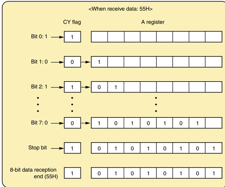
The receive data is saved to the A register and RRXDATA (RAM area) after 8-bit data reception ends. Furthermore, the CY flag value is reversed and saved to the X register and RRXFLAG (RAM area) as the receive status flag (0: normal reception, 1: framing error).
