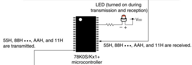
● Transmission test (received 8 units of data are transmitted)
