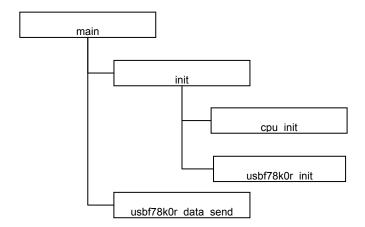
Figure 3-7 Calling Functions During the Processing for the USB Function Controller
