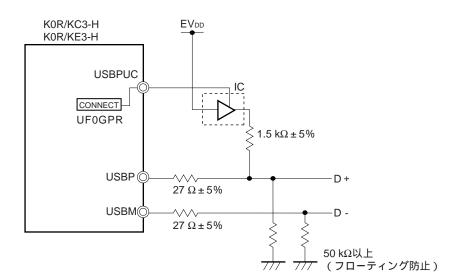
Figure 3-4 USB function controller Connection Example
