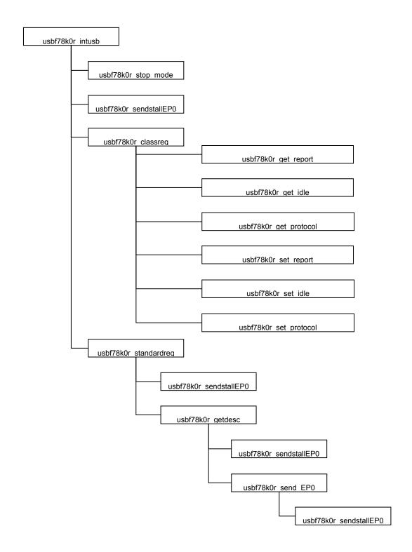
Figure 3-8 Calling Functions During the Processing for the USB HID class (1)
