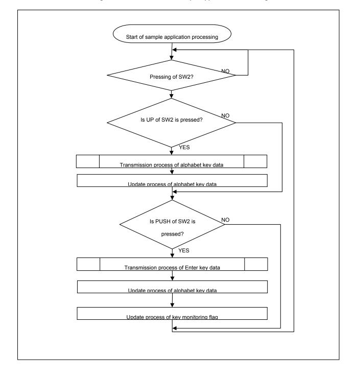
Figure 4-1 Flowchart for the Sample Application Processing
