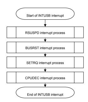
Figure 3-5 Process flowchart of INTUSB interrupt
