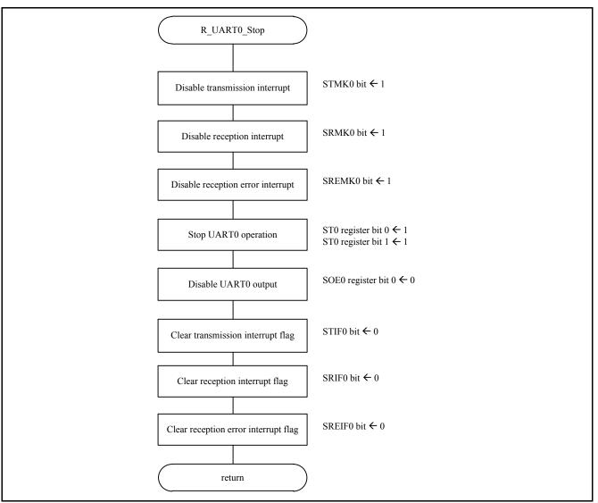
Figure 5.15 UART0 operation stop function
