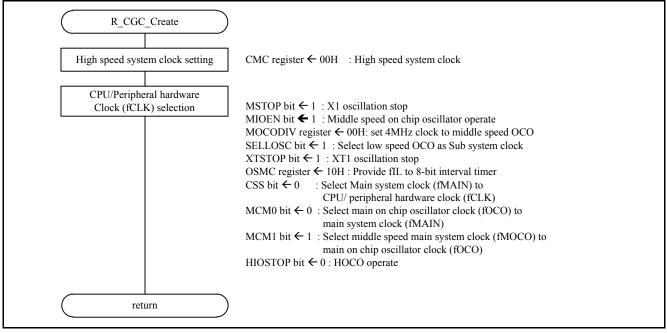
Figure 5.4 CPU clock initialization function
