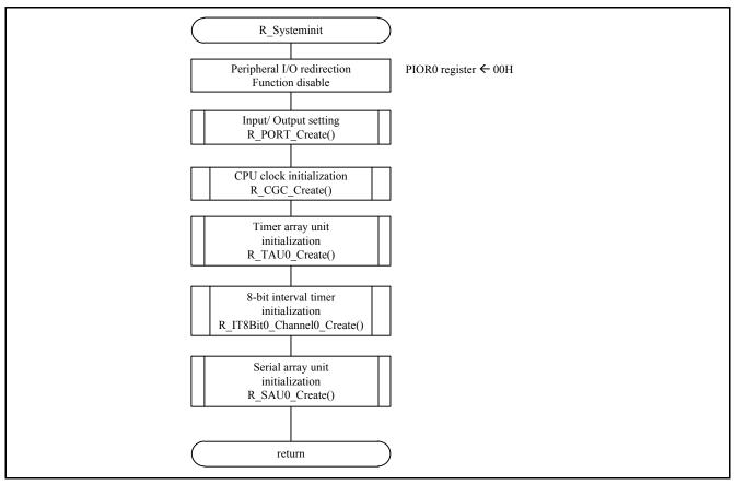
Figure 5.3 Peripheral function initialization function
