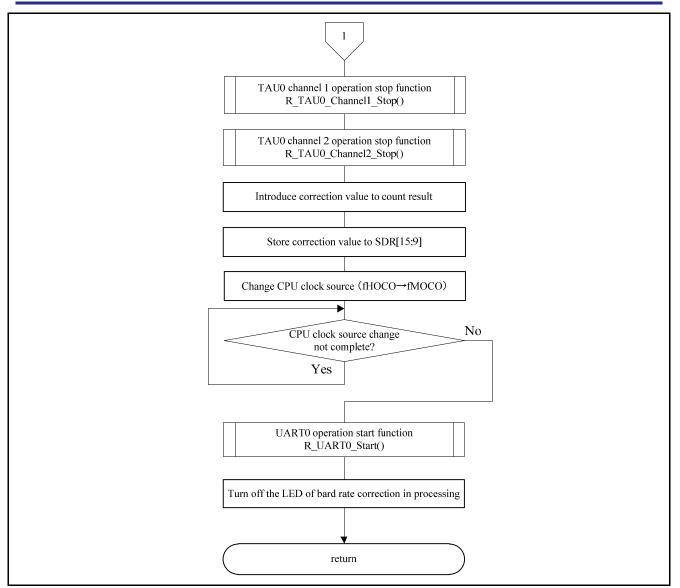
Figure 5.20 8-bit interval timer interrupt function (2/2)
