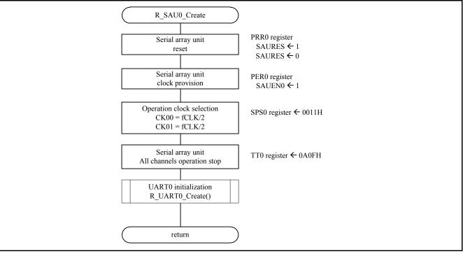
Figure 5.7 Serial array unit initialization function
