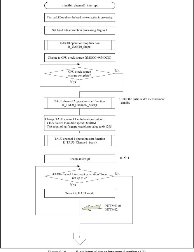
Figure 5.19 8-bit interval timer interrupt function (1/2)
