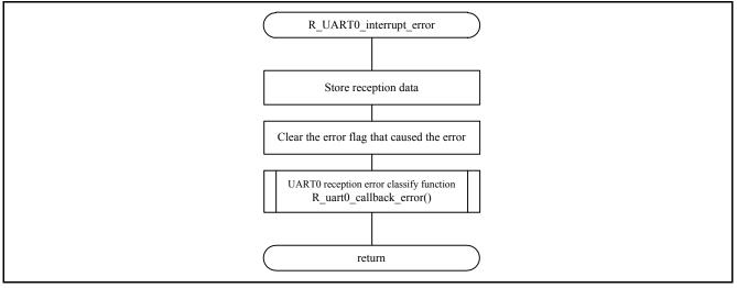
Figure 5.17 UART0 reception error interrupt function
