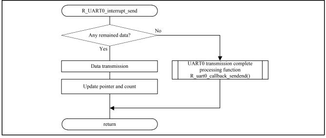
Figure 5.18 UART0 transmission complete interrupt function
