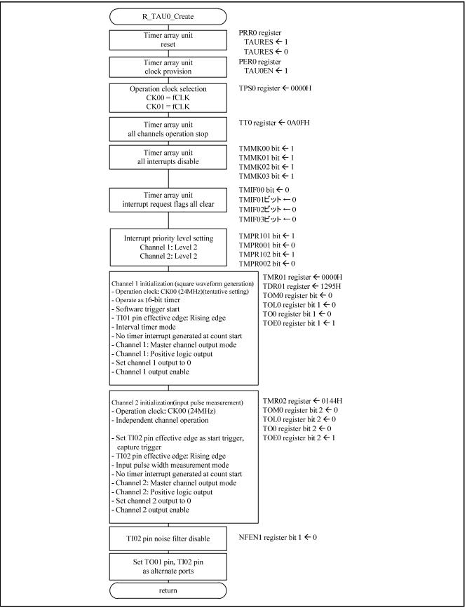
Figure 5.5 Timer array unit initialization
