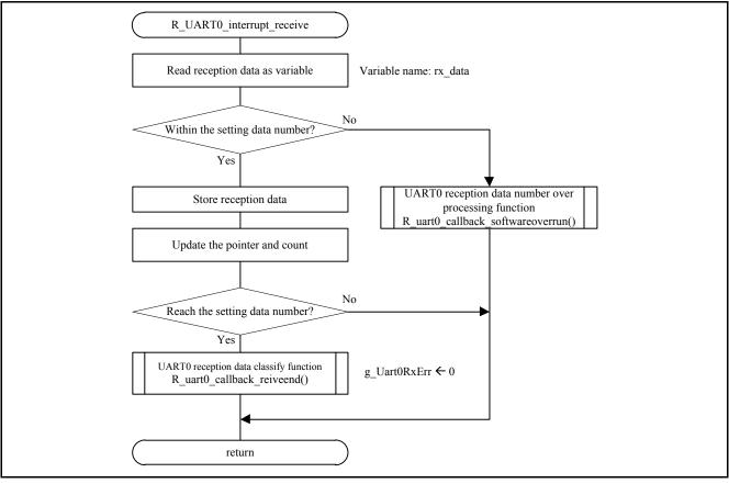
Figure 5.16 UART0 reception complete interrupt function
