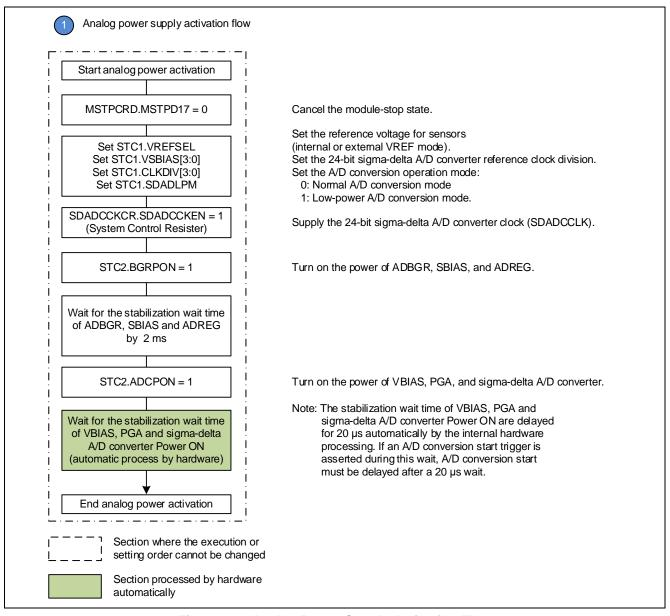
Figure 26. Analog Power Supply Activation Flow
