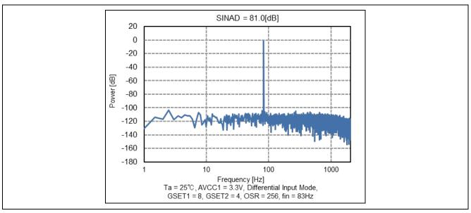
Figure 17. Power versus Frequency ( $G_{SET1} = 8$ ,  $G_{SET2} = 4$ , OSR = 256)
