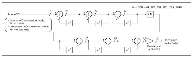
Figure 5. Digital Filter Block Diagram
