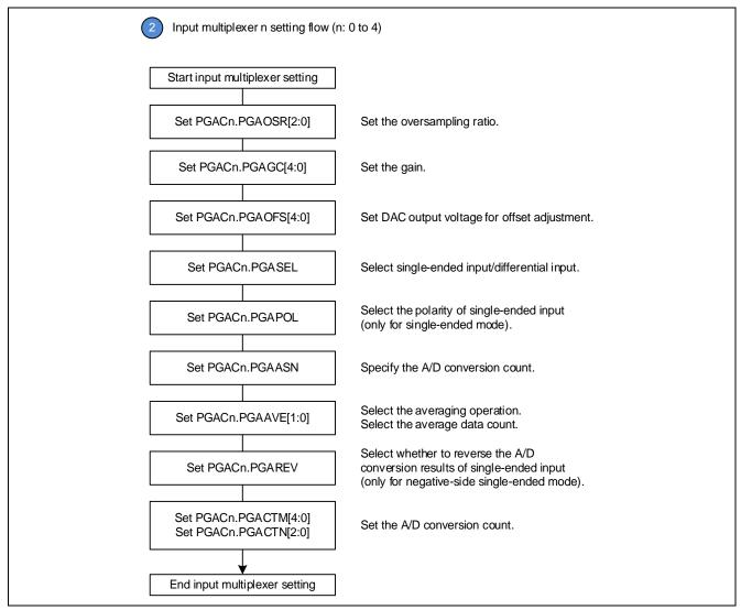
Figure 27. Input Multiplexer Setting Flow
