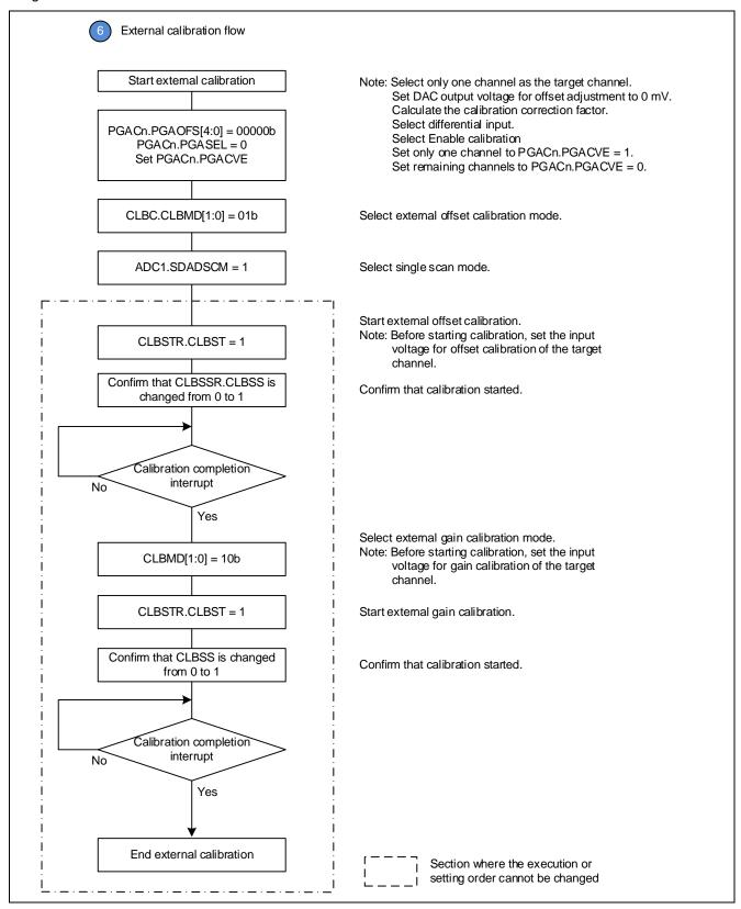
Figure 31. External Calibration Flow
