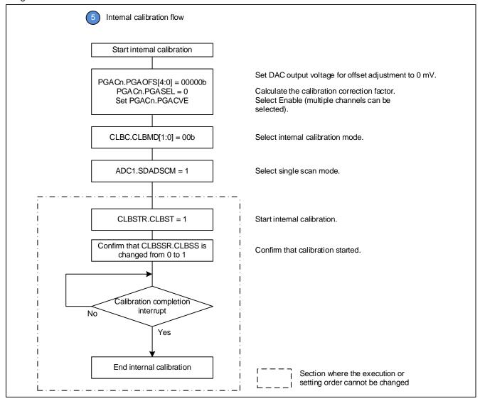
Figure 30. Internal Calibration Flow
