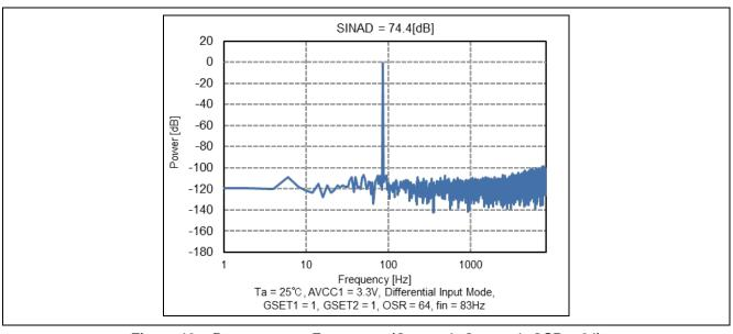
Figure 13. Power versus Frequency ( $G_{SET1} = 1$ ,  $G_{SET2} = 1$ , OSR = 64)
