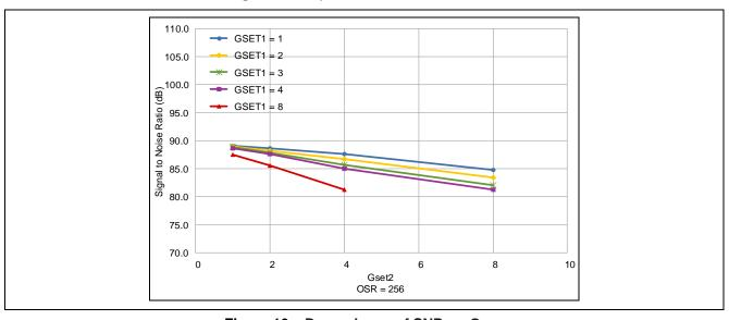
Figure 10. Dependence of SNR on  $G_{\text{SET2}}$
