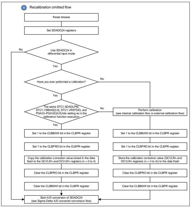
Figure 32. Recalibration Omitted Flow
