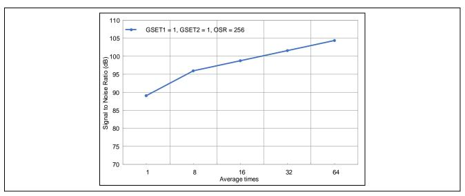
Figure 19. SNR versus Average Times
