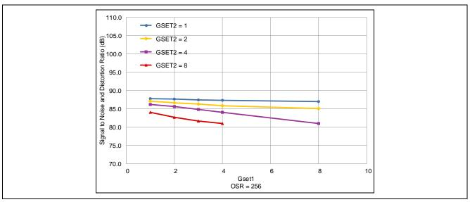
Figure 11. Dependence of SINAD on G<sub>SET1</sub>
