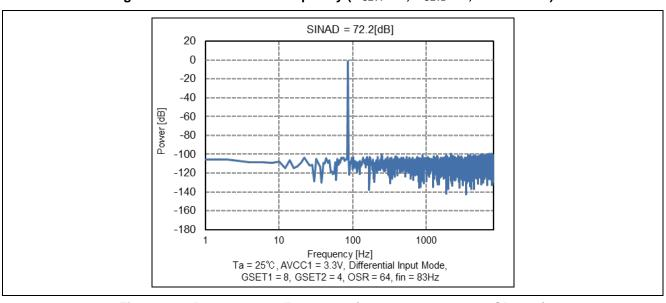
Figure 16. Power versus Frequency (G<sub>SET1</sub> = 8, G<sub>SET2</sub> = 4, OSR = 64)
