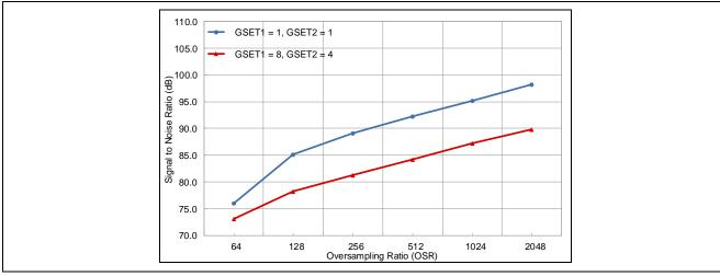
Figure 7. SNR versus OSR
