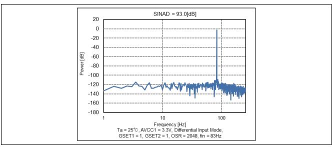
Figure 15. Power versus Frequency (G<sub>SET1</sub> = 1, G<sub>SET2</sub> = 1, OSR = 2048)
