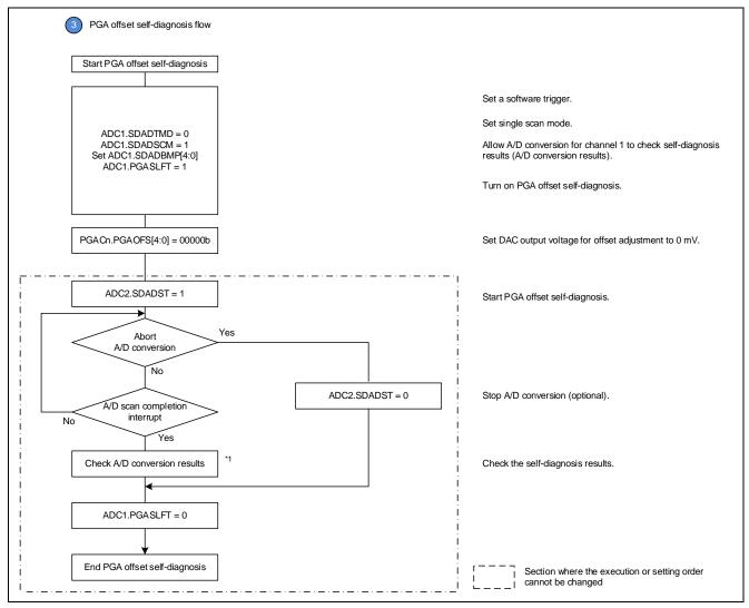
Figure 28. Self-diagnosis Flow for PGA Offset
