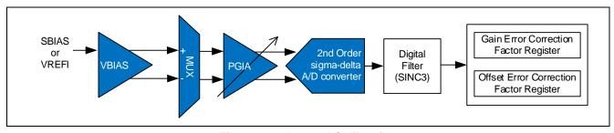
Figure 23. Internal Calibration
