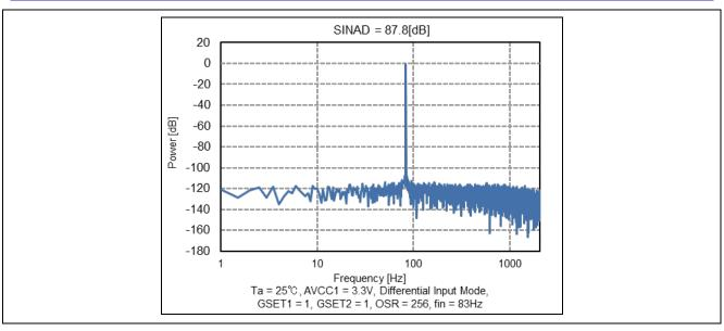
Figure 14. Power versus Frequency ( $G_{SET1} = 1$ ,  $G_{SET2} = 1$ , OSR = 256)
