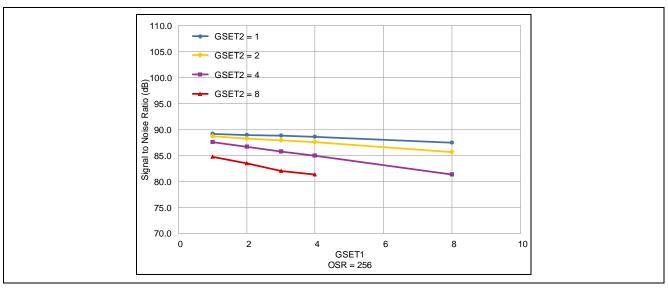
Figure 9. Dependence of SNR on G<sub>SET1</sub>
