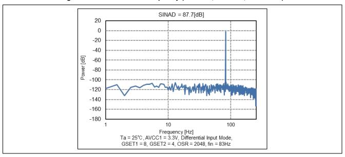
Figure 18. Power versus Frequency (G<sub>SET1</sub> = 8, G<sub>SET2</sub> = 4, OSR = 2048)
