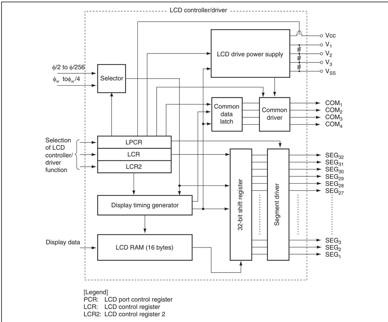
Figure 2.1 Block Diagram of LCD Controller/Driver
