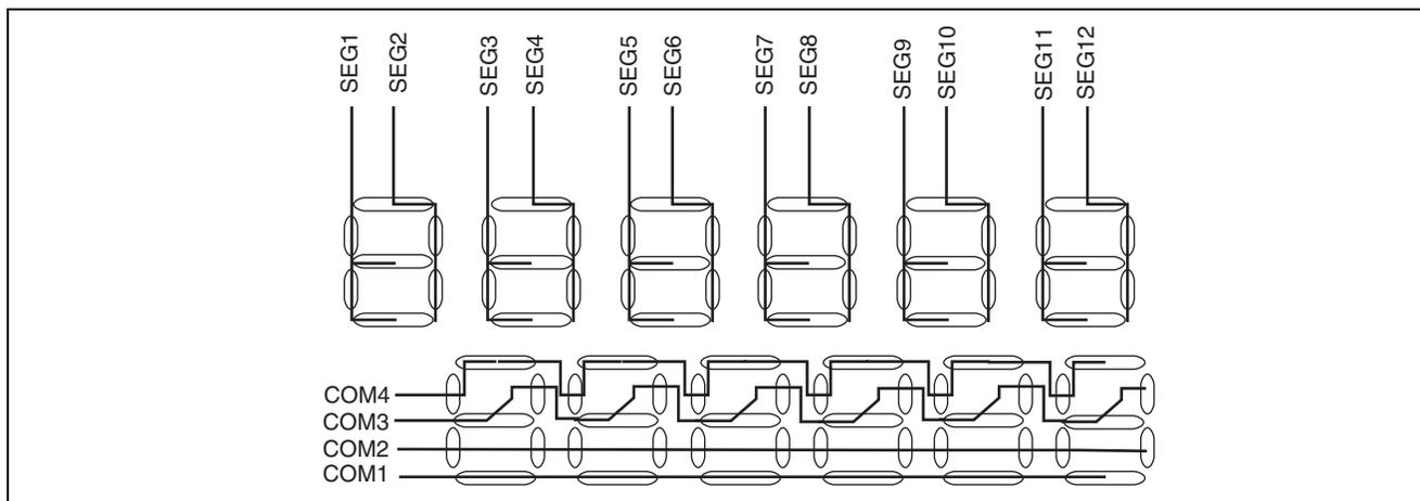
**Figure 2.2 Connections of Segment Signals and Common Signals for the 6-Digit 7-Segment LCD Used in this Sample task**
