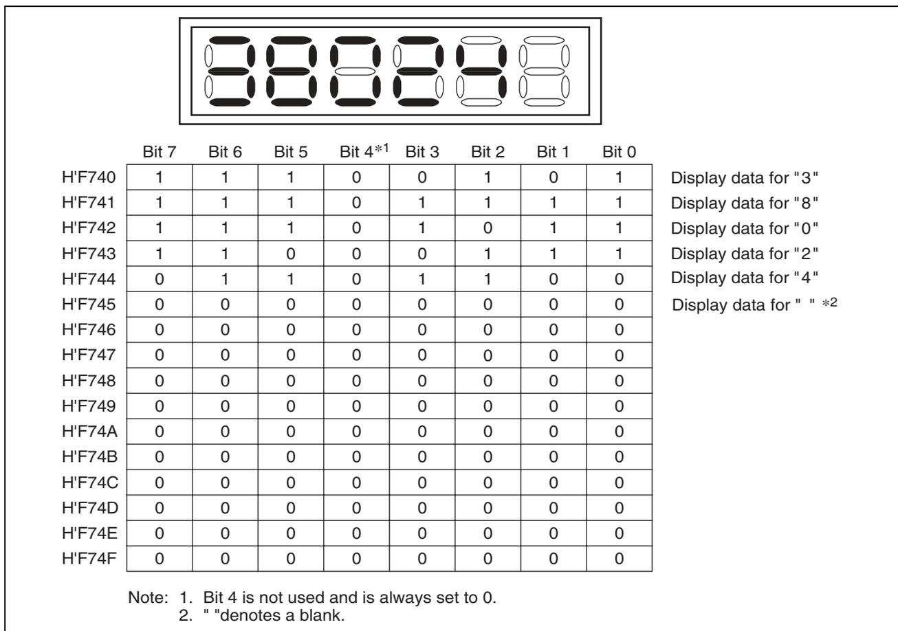
**Figure 2.4 Relation between LCD Display and LCD RAM Settings**
