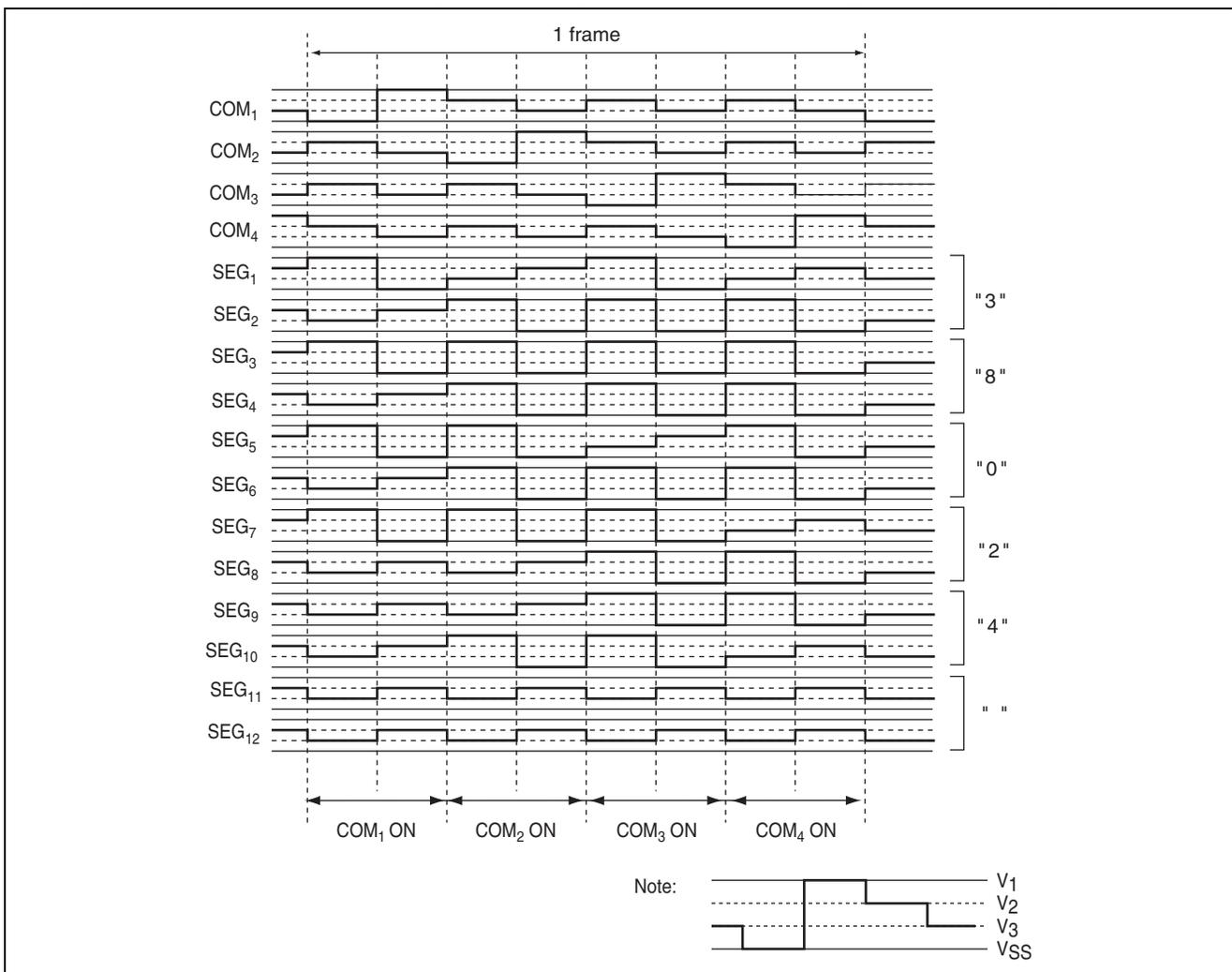
Figure 3.1 Waveforms of Segment Drive Signals
