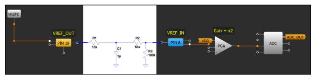
Figure 13 shows how a voltage divider connected to the filter in Figure 8 compensates for this difference. In this case, the PGA gain was set to x2. For simplicity, the resistor voltage divider could be replaced with a potentiometer for small adjustments.
