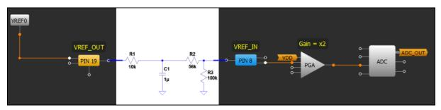
Figure 13. Voltage divider
